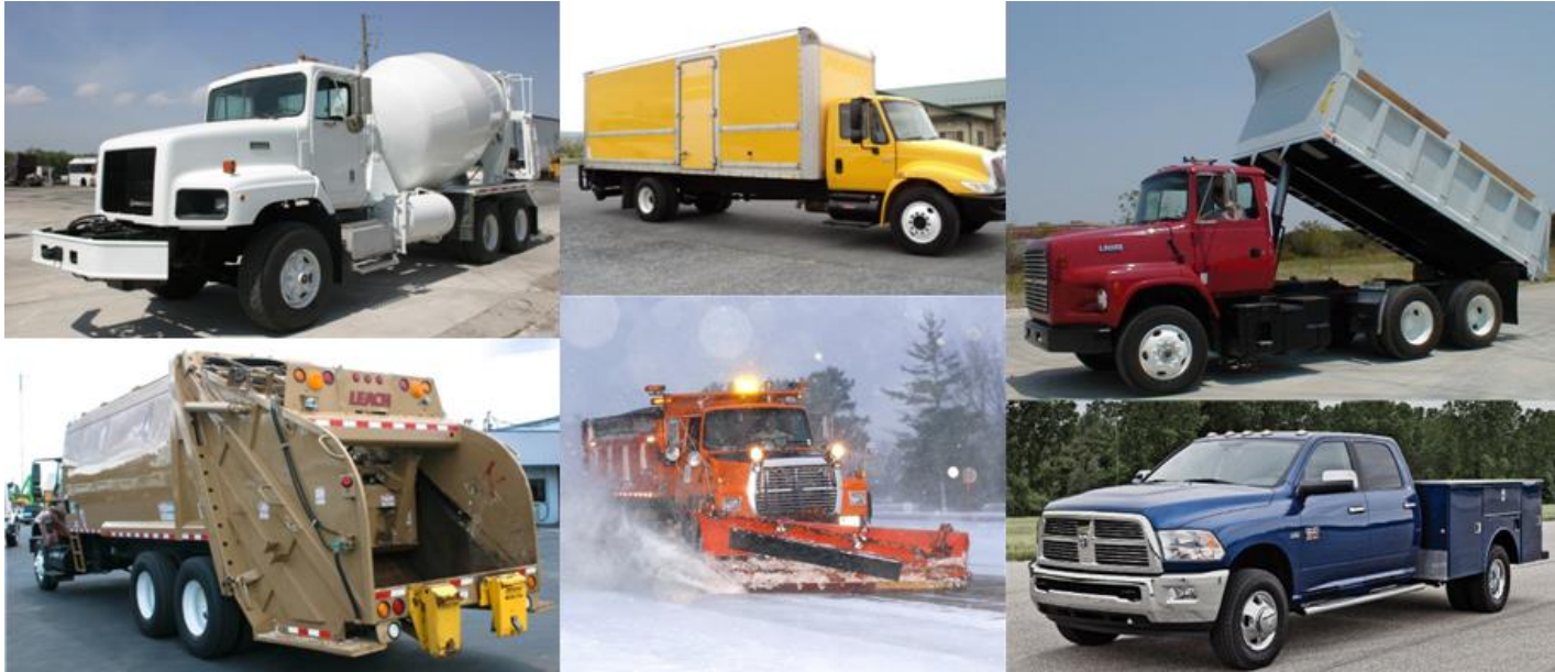
Figure 2. Different types of single-unit trucks.
