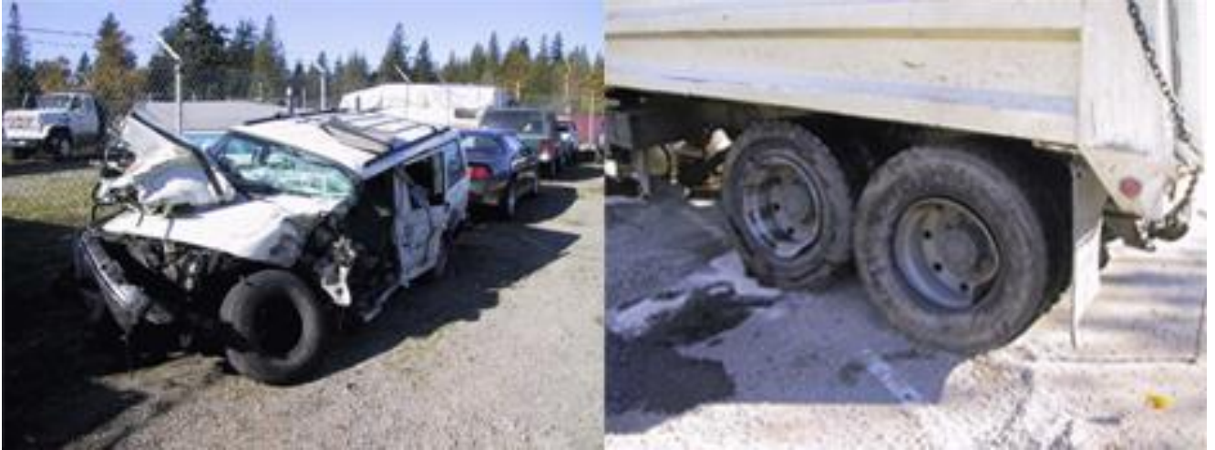
Figure 3. Photos of a Side Underride from Case 884005705, Large Truck Crash Causation Study.
