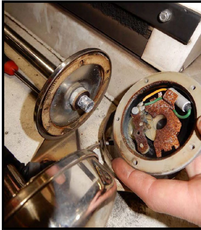
Figure 5. Internal components of a nonworking horn trumpet.
