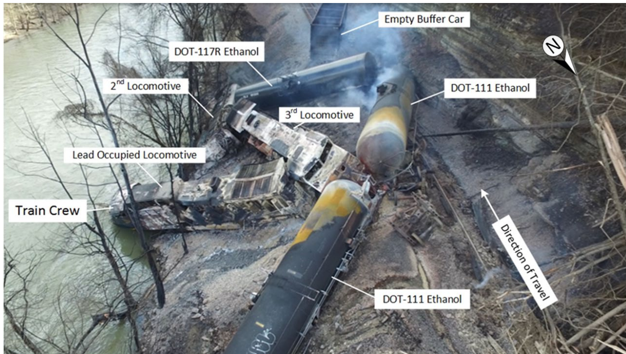
Figure 1. Derailment scene. (Photograph courtesy of Pike County Office of Emergency Management with overlay annotations by the National Transportation Safety Board.)
