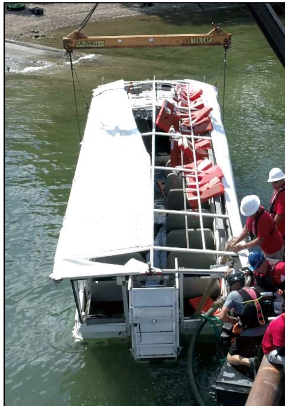
Figure 5. Torn canopy of the Stretch Duck 7 found during recovery operations.
