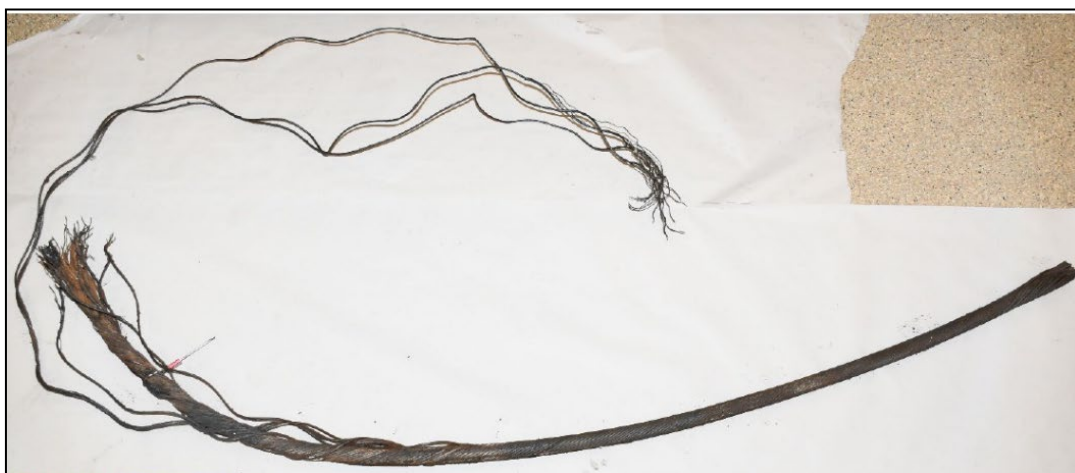
Figure 7. Thorco Basilisk parted hoisting wire rope (crane side of fracture). (Source: Engineering Systems Inc)
