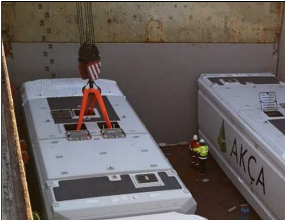
Figure 4. Exemplar Nordex Delta 4000 wind turbine nacelle in another vessel's cargo hold rigged in accordance with manufacturer-recommended guidance. (Source: Nordex)
