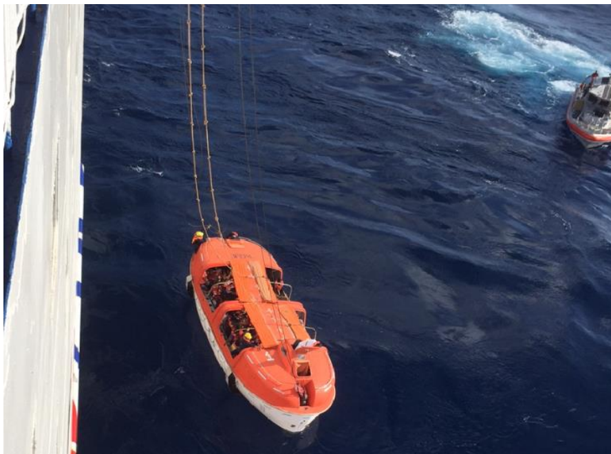
Figure 7. Lifeboat no. 1 in the water and unable to open the release hooks, about 0825. (Photo provided to Coast Guard by a Caribbean Fantasy passenger)
