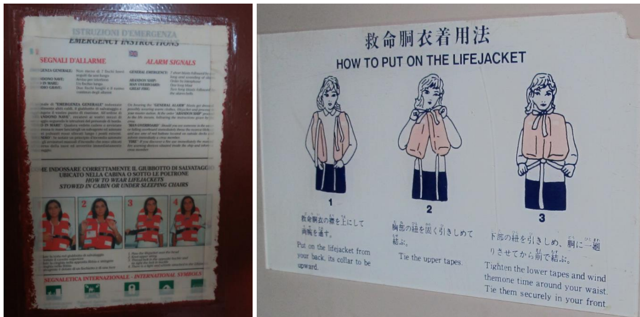
Figure 27. Left: Emergency instruction sign in English and Italian on the back of a deck 6 cabin door. Note the masking tape covering the outer edges of the emergency instructions. Right: Lifejacket donning instruction sign in English and Japanese found on deck 6 near fire locker no. 2. The instructions were for lifejacket types not carried on board at the time of the accident.
