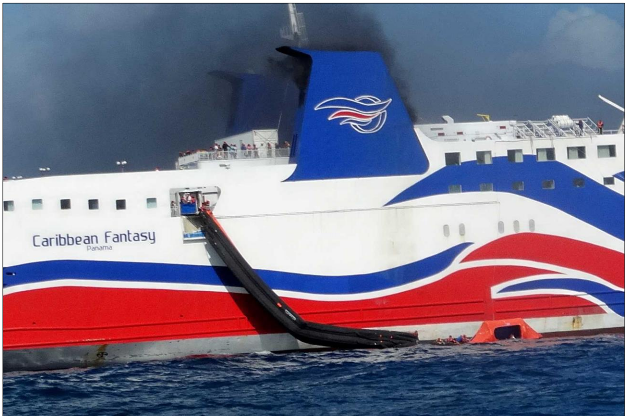
Figure 25. Caribbean Fantasy starboard-side MES deployed at about a 54-degree angle to the waterline, about 0923 on the morning of the accident. (Photo by US Coast Guard)
