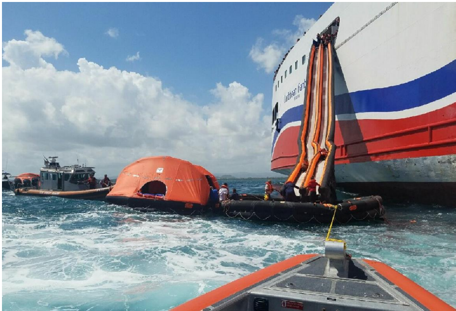
Figure 11. Bow of Coast Guard small boat, about 1012, as it began to pull the starboard-side MES platform forward, with another small boat holding a liferaft to the platform. Two evacuees with lifejackets are on the slide, while many others are looking over the ship's side from the deck above the MES embarkation landing. (Photo by Coast Guard)
