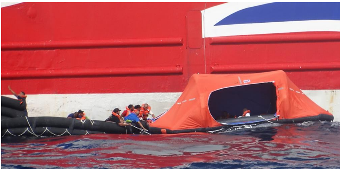
Figure 9. Liferaft at the starboard-side MES platform with the main access opening facing away from the platform, about 0923. (Photo by Coast Guard)
