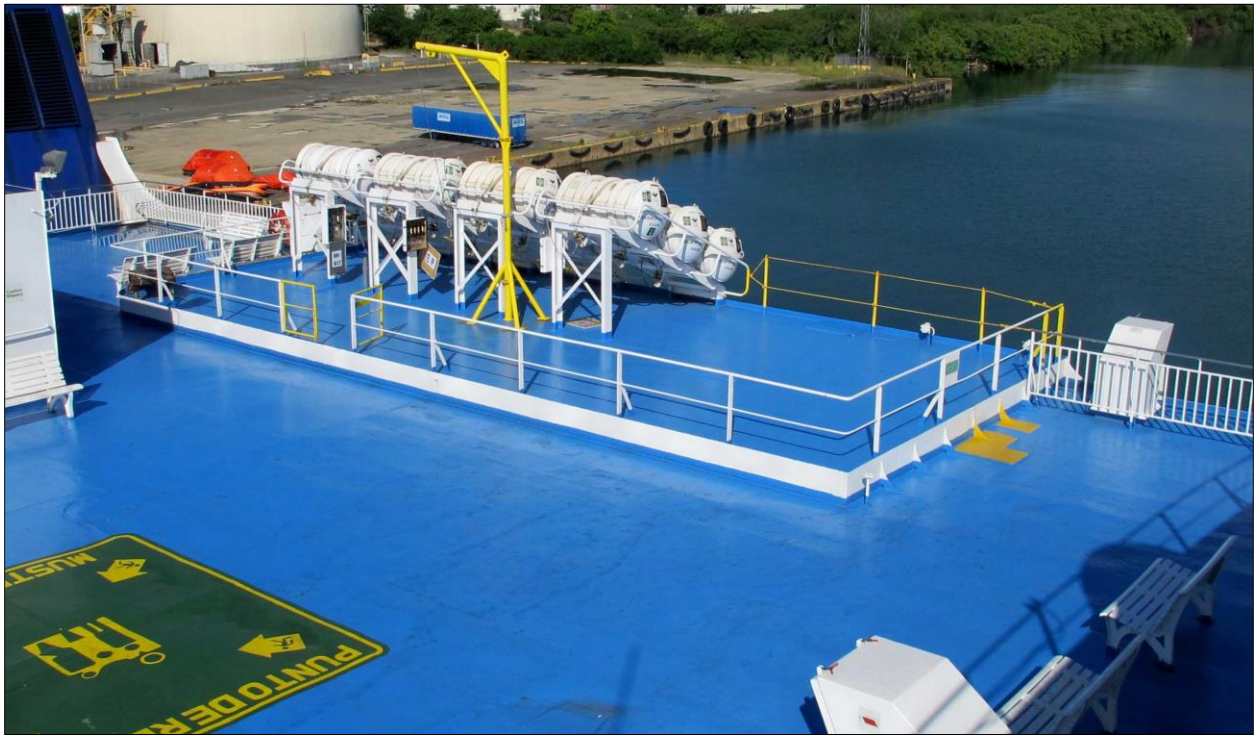
Figure 24. Postaccident photo of the portside liferaft containers and storage racks on board the Caribbean Fantasy .
