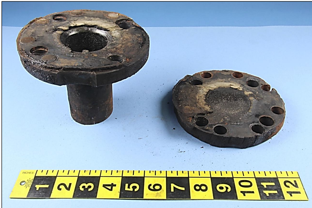
Figure 16. Fuel supply line end flange and gasket material, left, and blanking plate, right.
