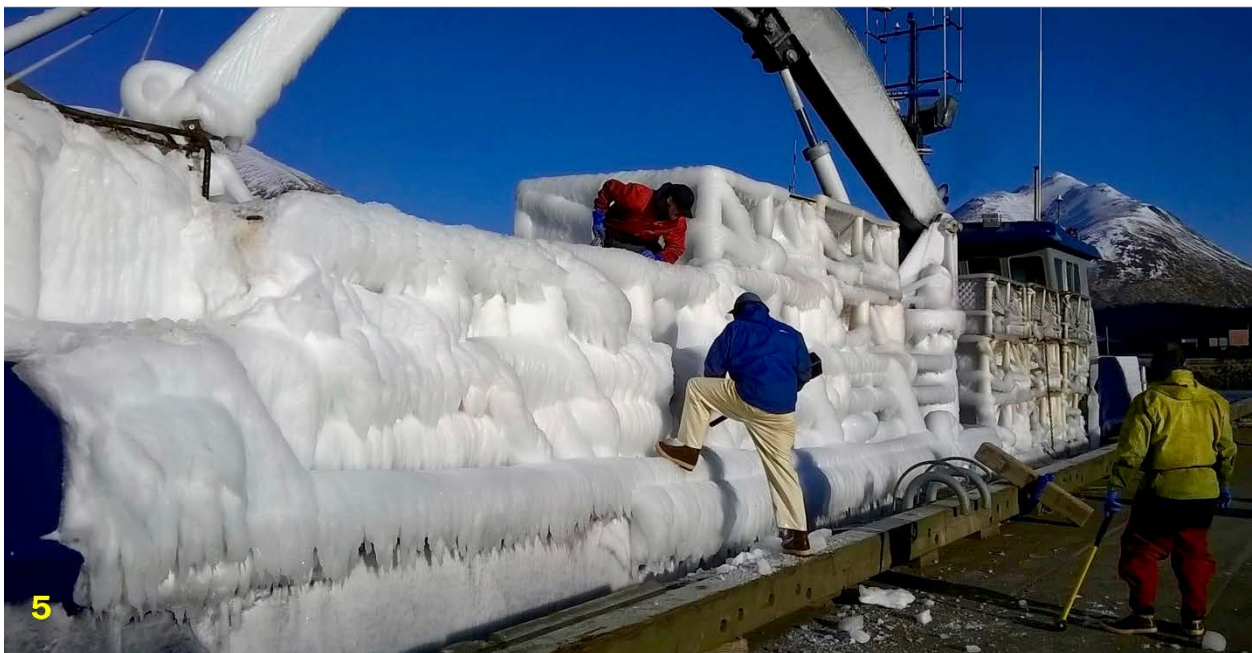
(1, 2, and 3) Polar Sea : ice covers the decks and anchor chain during the vessel's transit to St. Paul Island on February 10 and remains on the wheelhouse while it was docked there the following day. (4) Bering Rose : accumulation of ice on deck aft of the wheelhouse during the early hours of February 11. (5) Sandra Five : while in King Cove on February 12, crewmembers examine the ice that accumulated during their transit from St. Paul Island.
