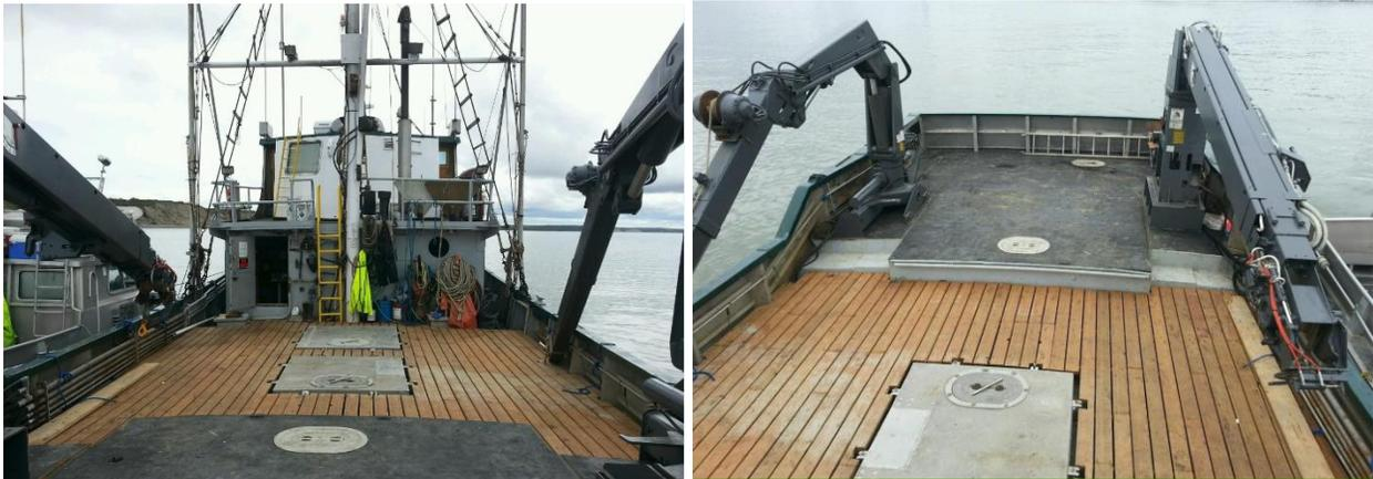
**At left is the aft main deck of the *Ambition*, viewed from the stern, showing rectangular bolted hatches for the forward and aft fish holds with access hatches inset. At right is the aft deck, viewed from the deckhouse, showing access hatches to the lazarette and potable-water tank.**
