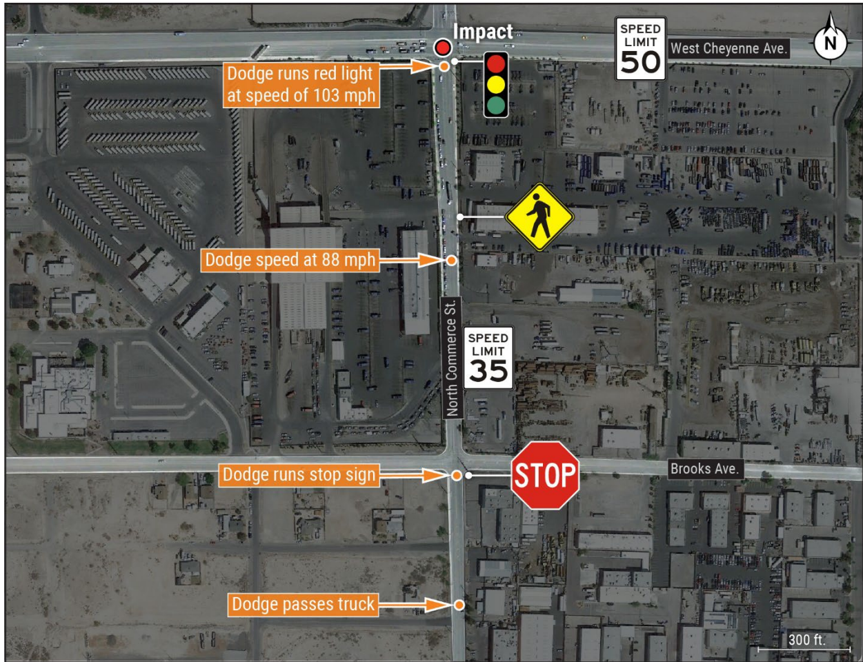
Figure 2. Locations of Dodge driver actions leading up to the crash. Traffic signs and signals along North Commerce Street are also shown. (Source: Google Earth; annotations added by the National Transportation Safety Board [NTSB])
