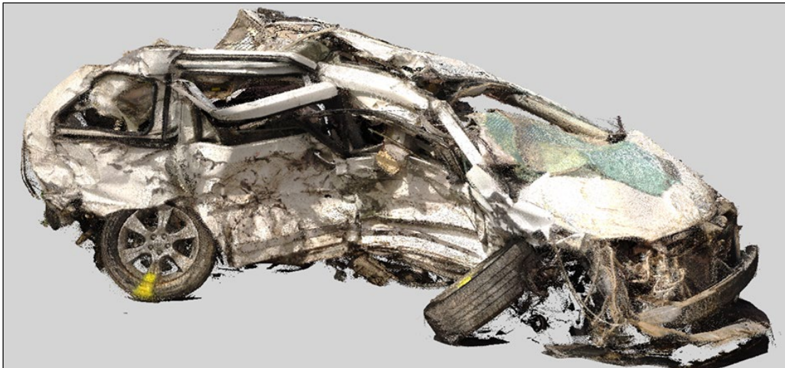
Figure 7. 3D laser scan showing damage to the Toyota Sienna (passenger side view).
