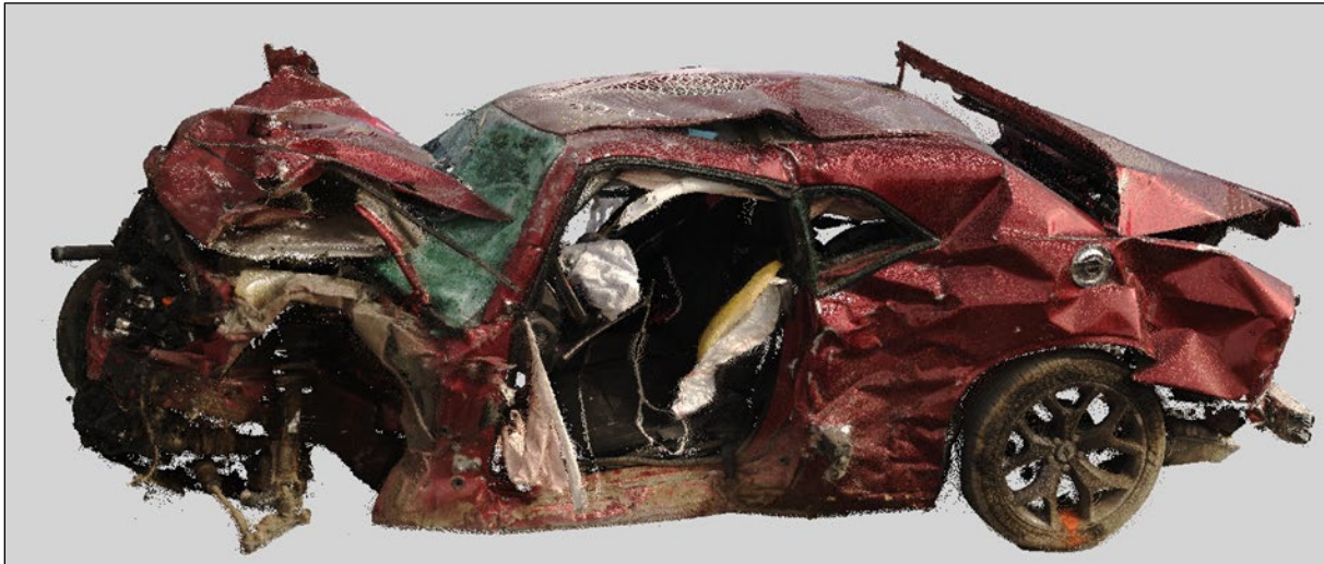
Figure 6. 3D laser scan showing damage to the Dodge Challenger. The view is from the driver's side, and the driver's door was removed during extrication of the driver.
