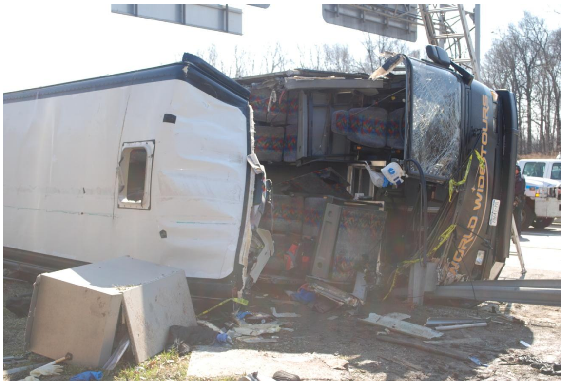
Figure 6. Roof separation due to intrusion of the vertical highway signpost poles.
