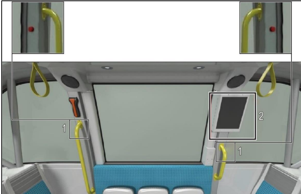
Figure 5. Rendering of shuttle interior showing locations of (1) emergency stop buttons (detailed in inset drawings) and (2) navigation touch screen. Emergency hammer (red) is shown in upper left. (Adapted from Navya owner’s manual)
