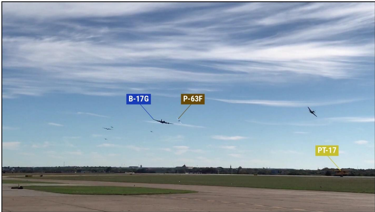
Figure 11. Video frame recorded 0.63 seconds before the collision showing the Bell P-63F in a left turn behind and off the left side of the Boeing B-17G. The revenue ride flight Boeing PT-17 is on the runway.
