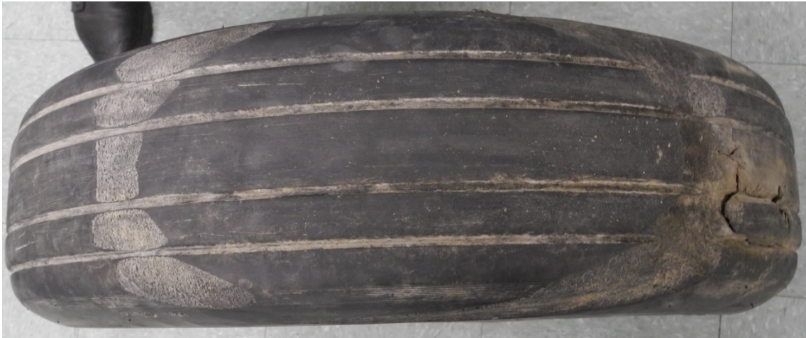
Figure 6. Additional worn area on the left outboard tire.
