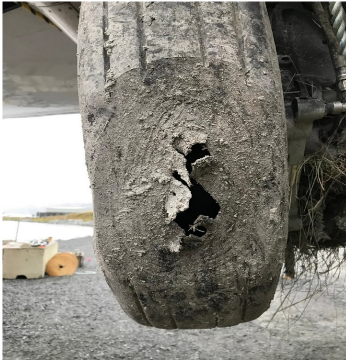
Figure 5. Worn area and hole in left outboard tire.
