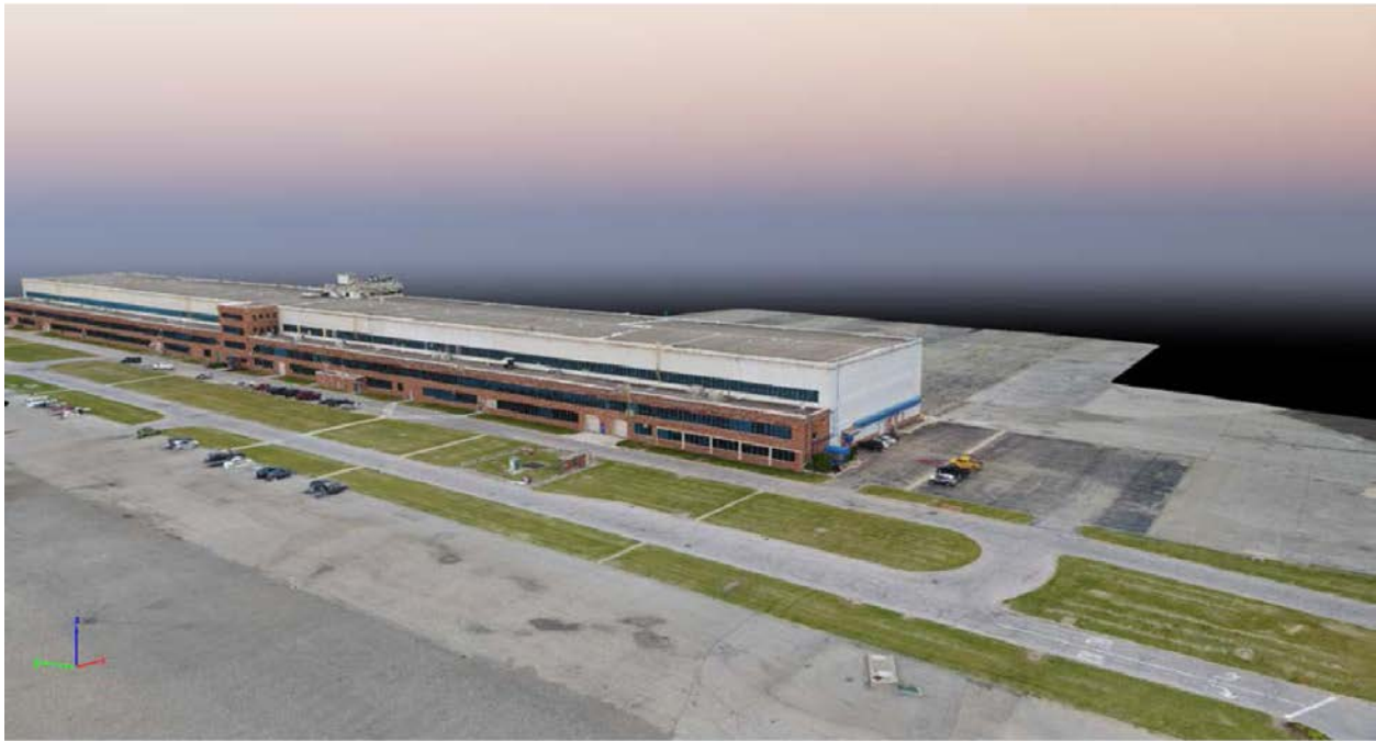
Figure 17. Screenshot of one view of the hangar 3-D model created from sUAS-captured imagery.
