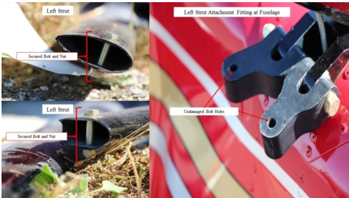
Figure 2: The left picture shows the left-wing strut attachment fitting ends, and the right picture shows the fuselage attachment fittings as found at the accident site.
