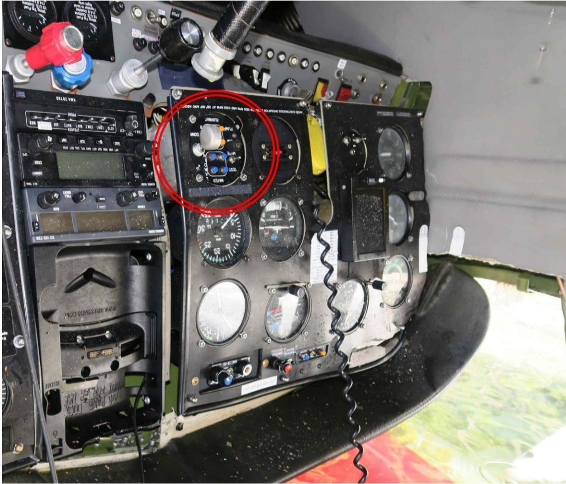
Figure 2. Landing gear control in “DOWN” position (Airplane upside down in water).
