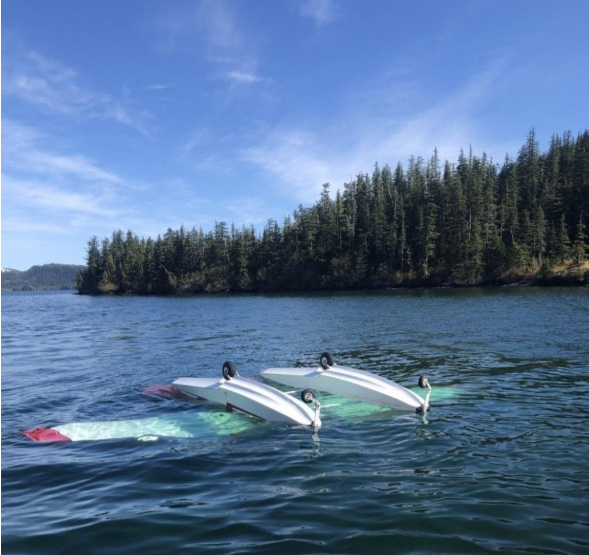
Figure 1. Airplane at the accident site with landing gear extended.
