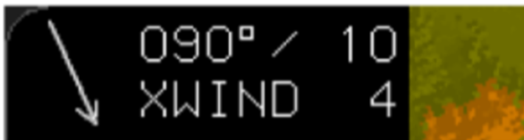
Figure 4. Chelton IDU calculated wind indication.
