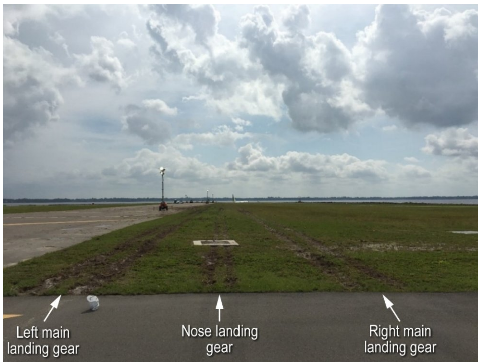
Figure 1. Photograph of tire marks from the accident airplane's landing gear
