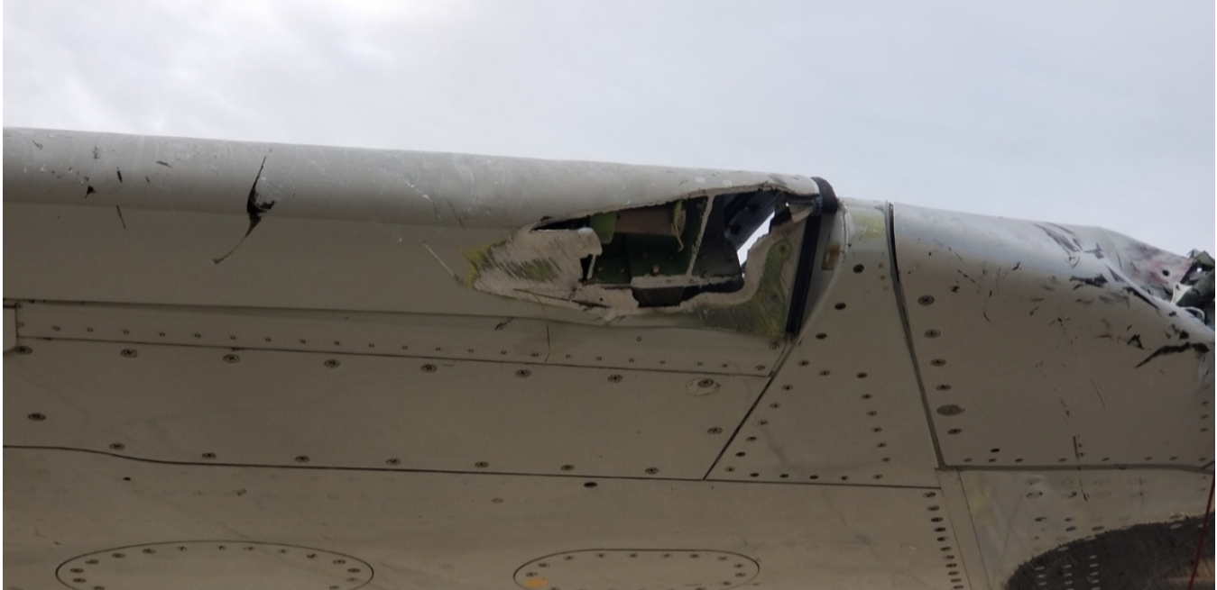
Figure 2. Scrape damage to underside of left wing slat (Source: American Airlines).
