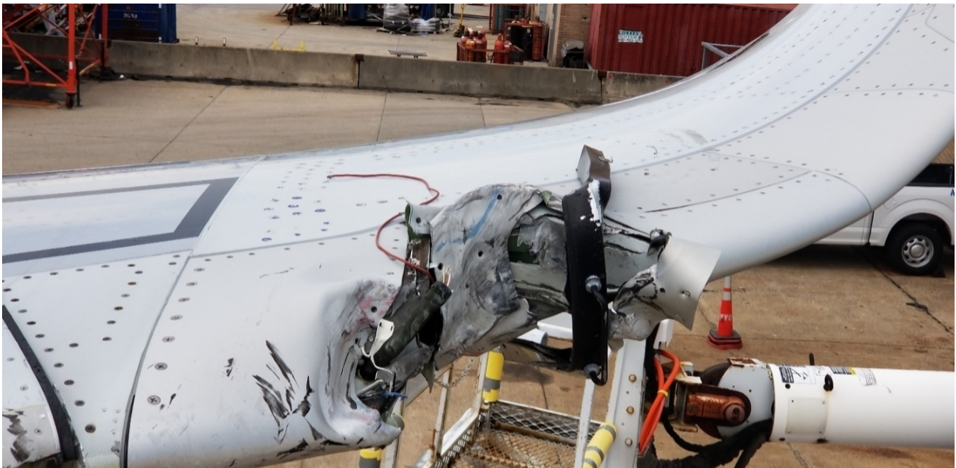
Figure 1. Left wingtip damage and portion of distance remaining marker support structure lodged in wingtip (Source: American Airlines).
