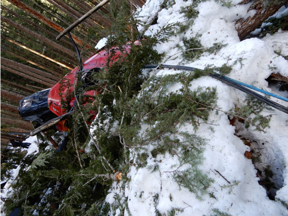
Figure 1. The helicopter at the accident site. A blue cargo line and two black hydraulic hoses can be seen running uphill to the grapple hook.
