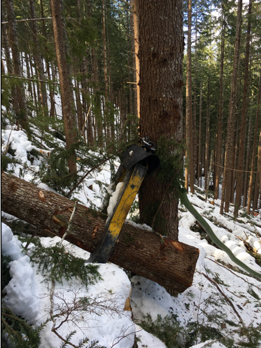
Figure 2. The grapple hook, attached to a log, and leaning against a standing tree. The cargo line and two hydraulic lines are contained in a green protective sheath and run downhill to the helicopter.
