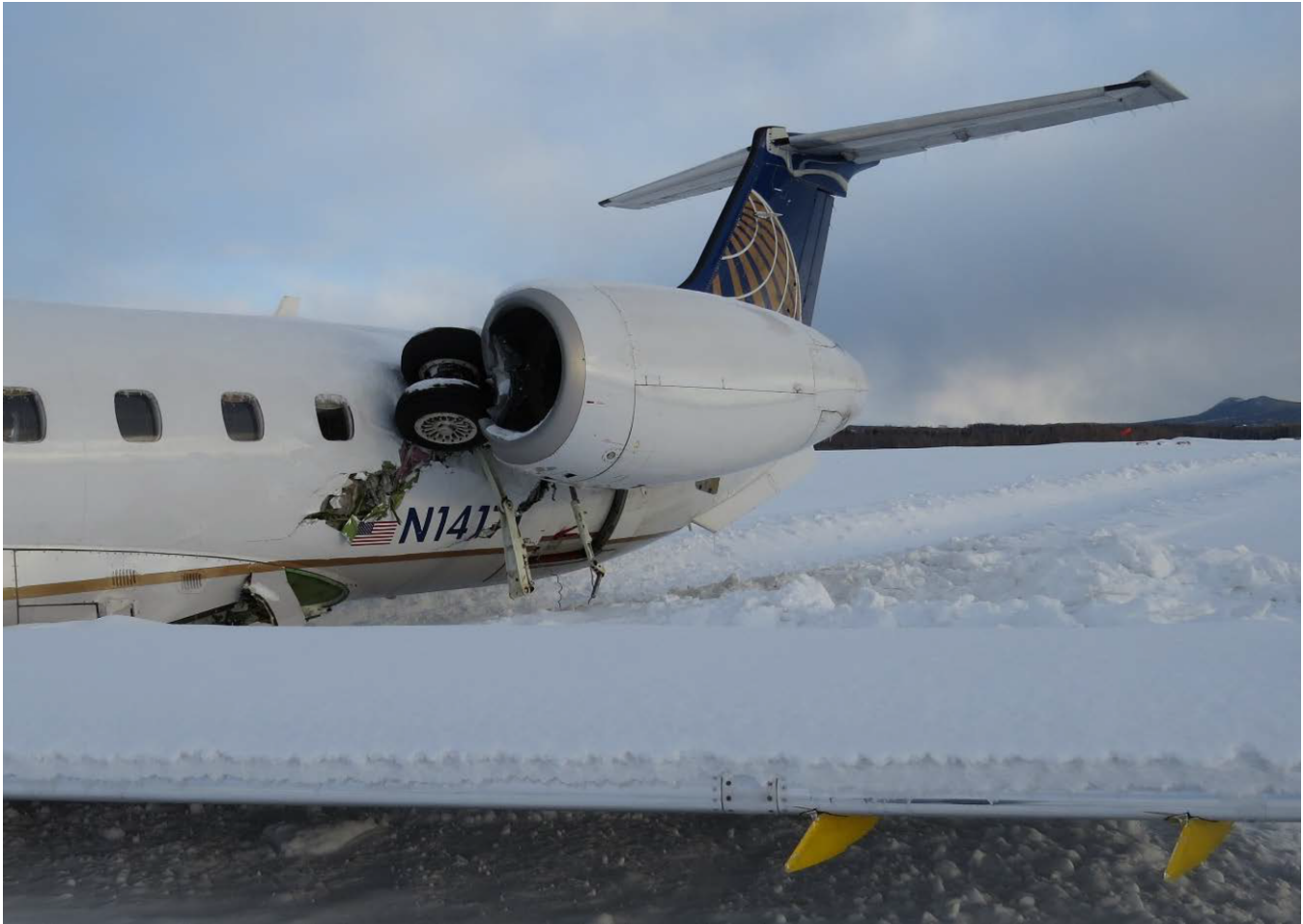
Figure 2: Left main landing gear lodged between left engine nacelle and the aircraft fuselage
