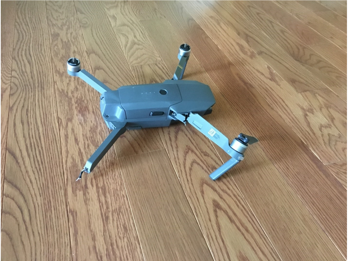
Figure 5 - Damaged Mavic Pro drone
