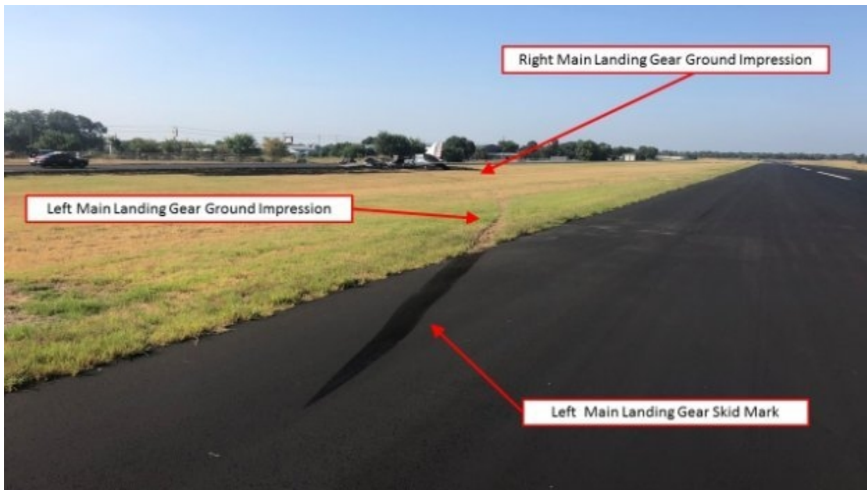
Figure 2. A photograph showing the left MLG wheel skid mark on the runway and the left MLG ground impressions left of the runway.
