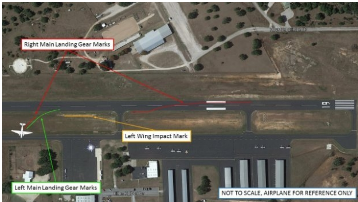
Figure 3. An overhead image of the right MLG wheel skid mark, the right and left MLG ground impressions, and the left-wing impact mark locations observed at the accident site.
