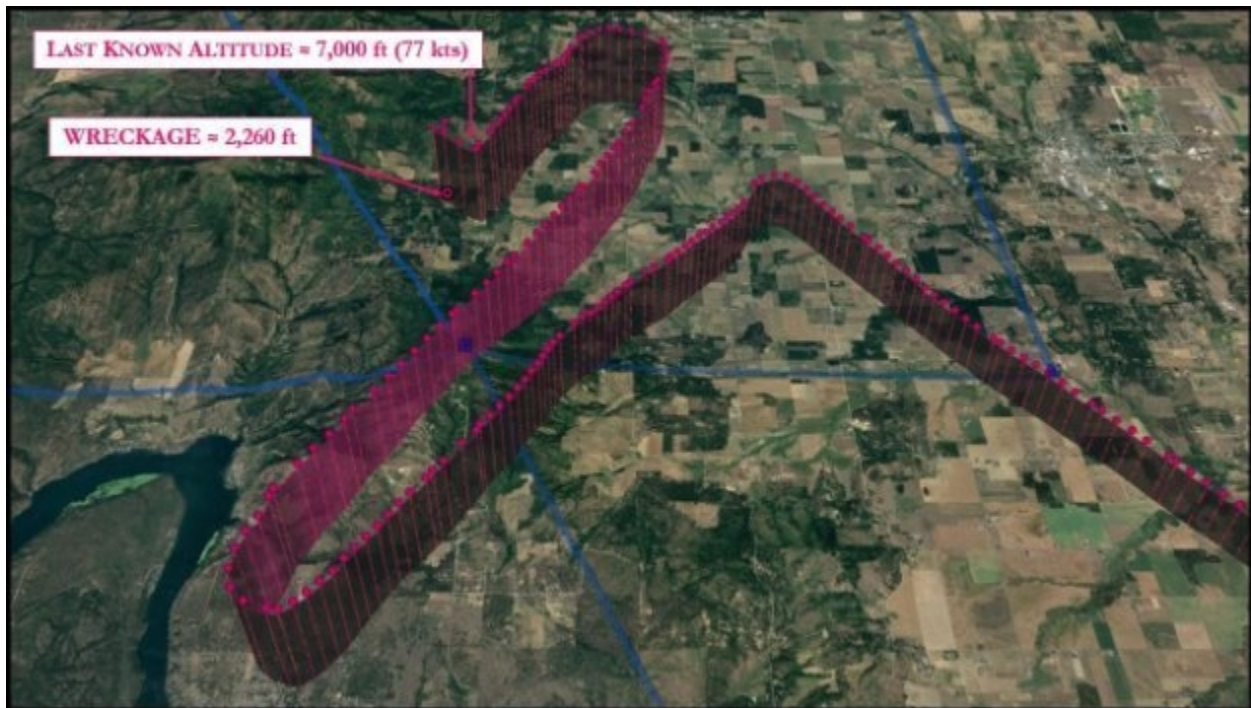
Figure 2: Radar Data Prior to Accident (showing altitude profile)
