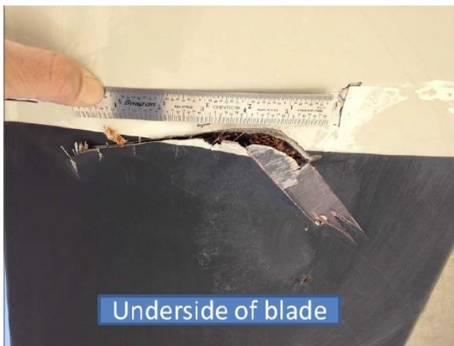
Figure 3 – Damaged Main Rotor Blade (Courtesy of Chevron)
