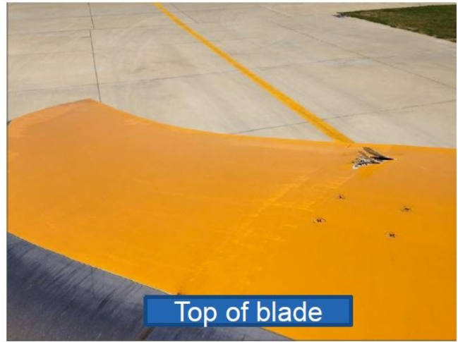
Figure 3 – Damaged Main Rotor Blade (Courtesy of Chevron)
