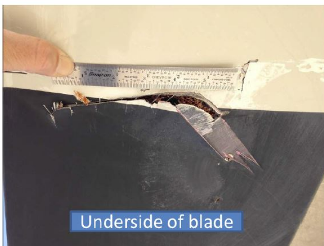
Figure 3 – Damaged Main Rotor Blade (Courtesy of Chevron)
