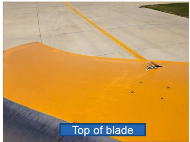
Figure 3 – Damaged Main Rotor Blade (Courtesy of Chevron)
