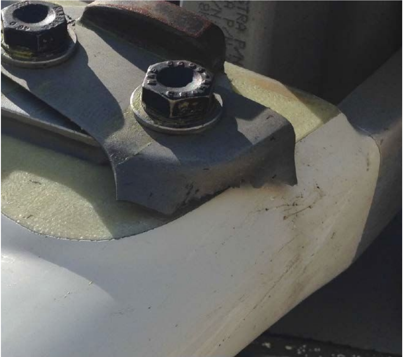
Figure 2 – Damaged Tail Rotor Erosion Shield Extension (Courtesy of Chevron)
