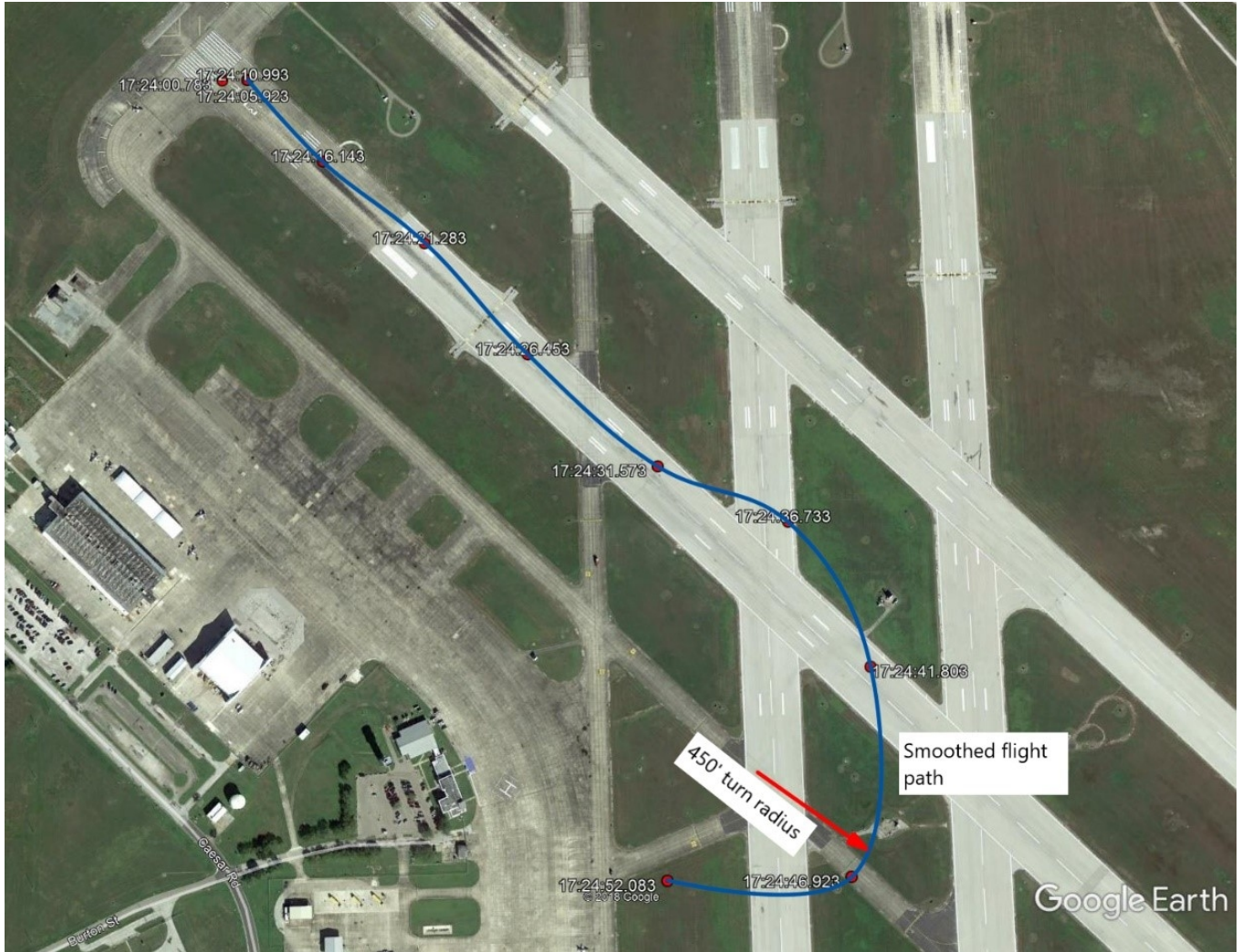
Figure 2. Overhead view of the airplane's ground track
