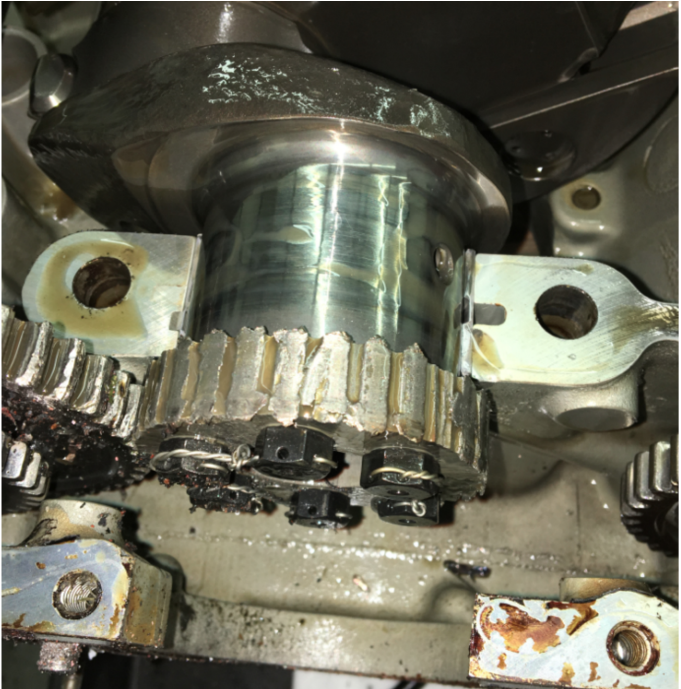
Figure 1. Crankshaft gear damage.
