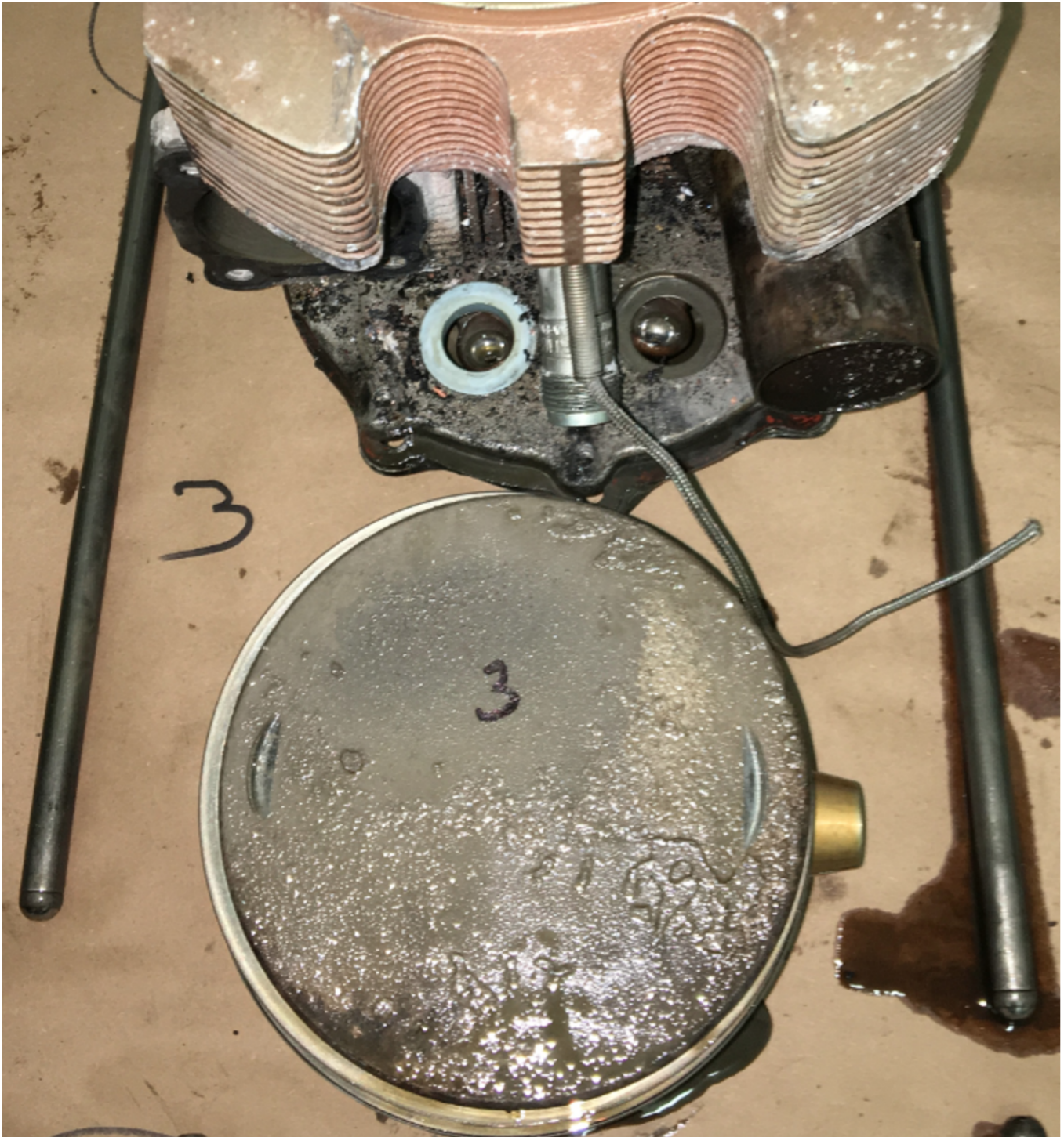
Figure 2. Piston No. 3 "scallop" impact marks from the valves at the 9:00 and 3:00 o'clock position. All 6 pistons exhibited similar signatures.
