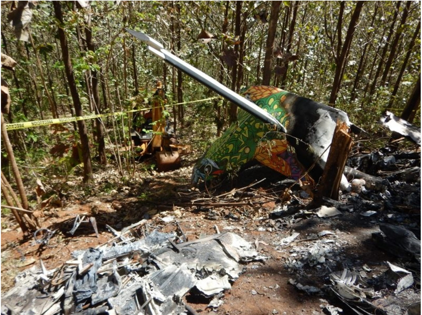
Figure 3 - View of the airplane's tail section at the accident site.
