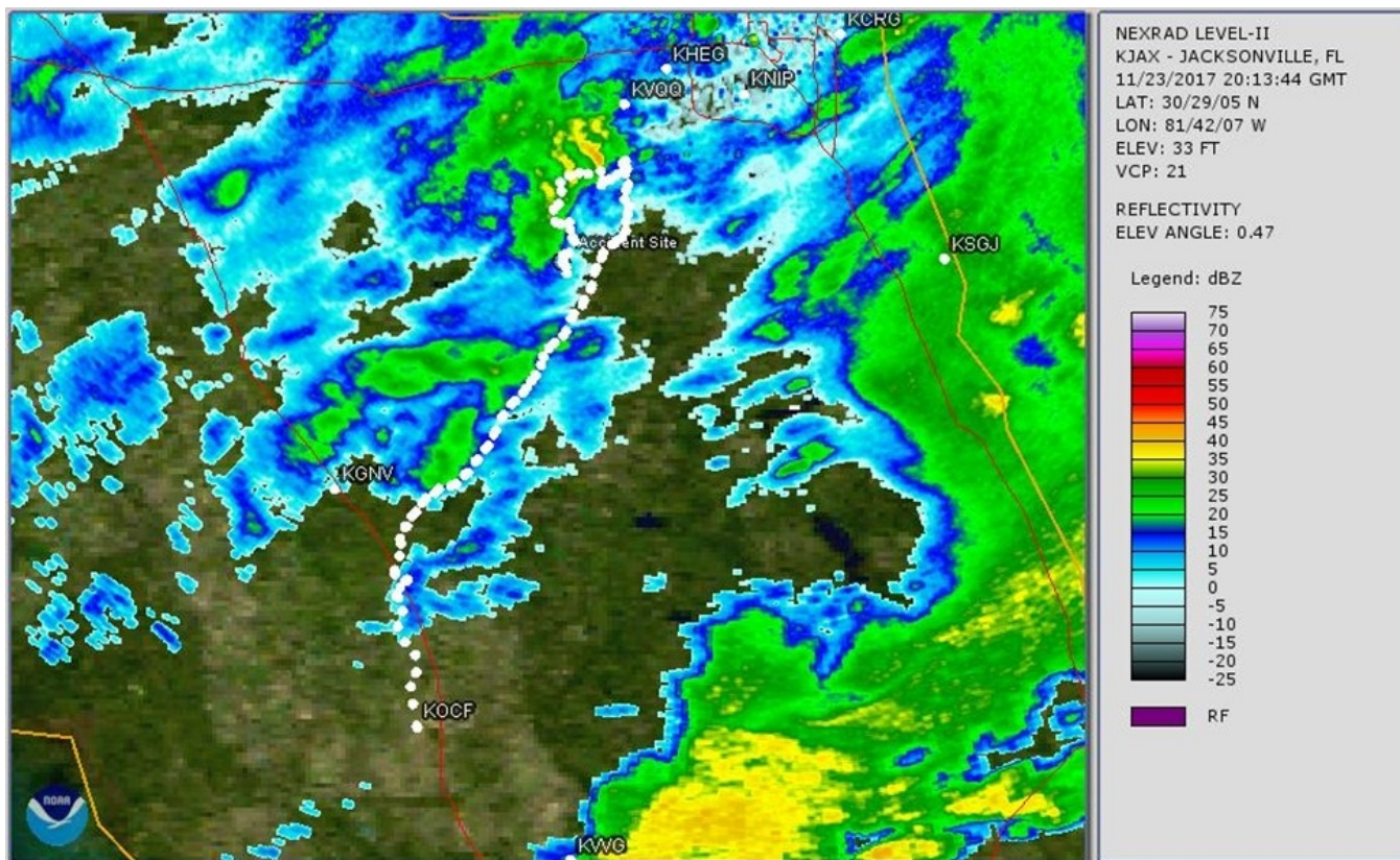
Figure 1. KJAX WSR-88D 0.5° base reflectivity image for 1513 with airplane's flight track of overlaid
