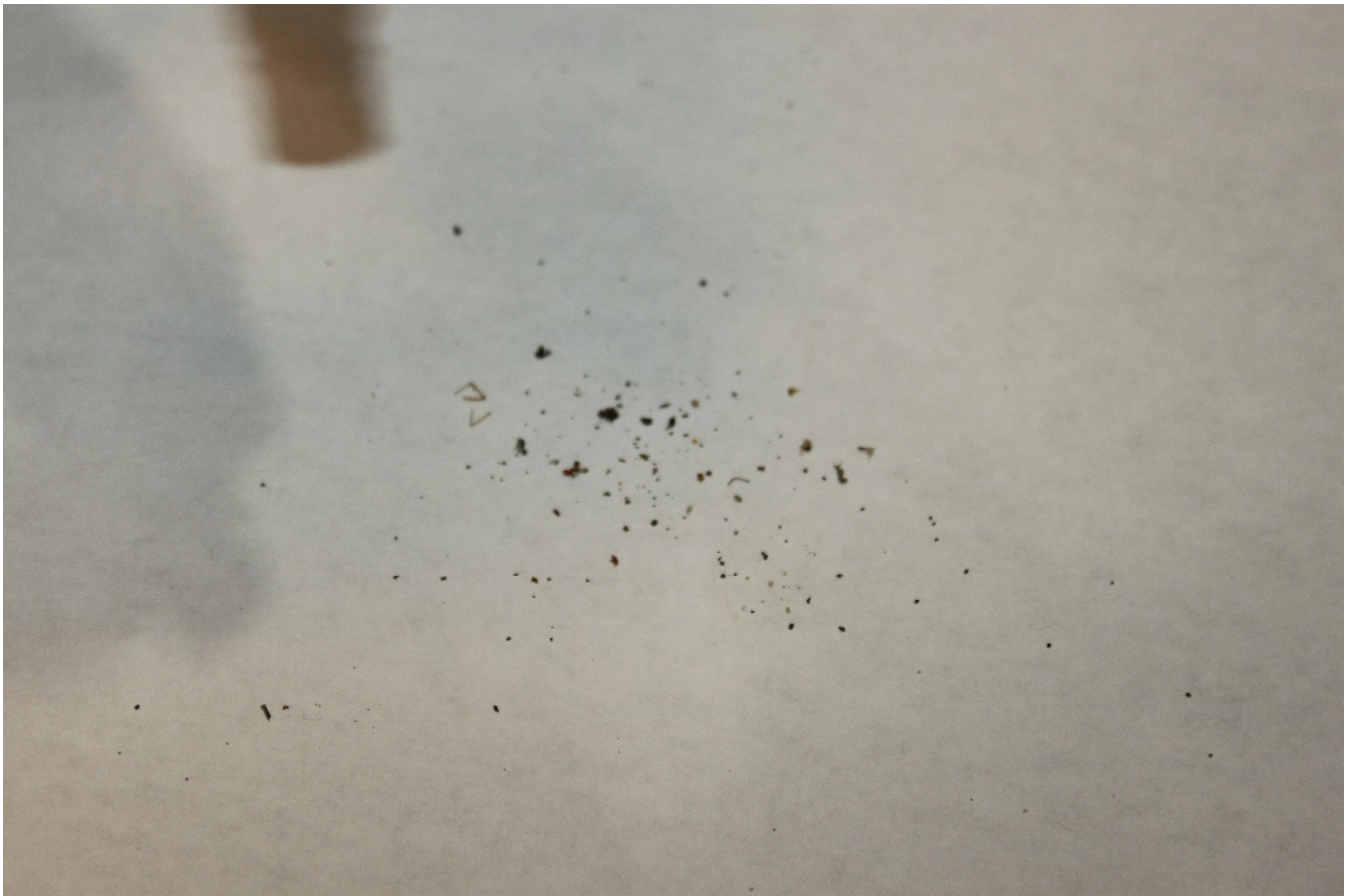
Fuel Servo Debris
