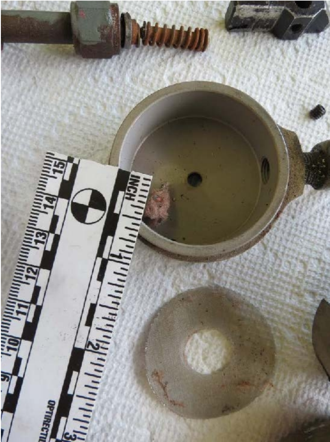
Figure 1-Debris discovered in the fuel selector.
