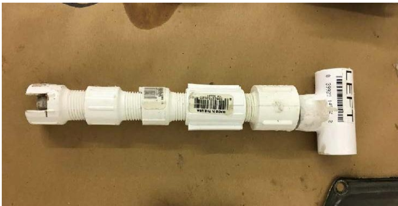
Figure 2-Homemade fuel selector tool after partial reassembly.
