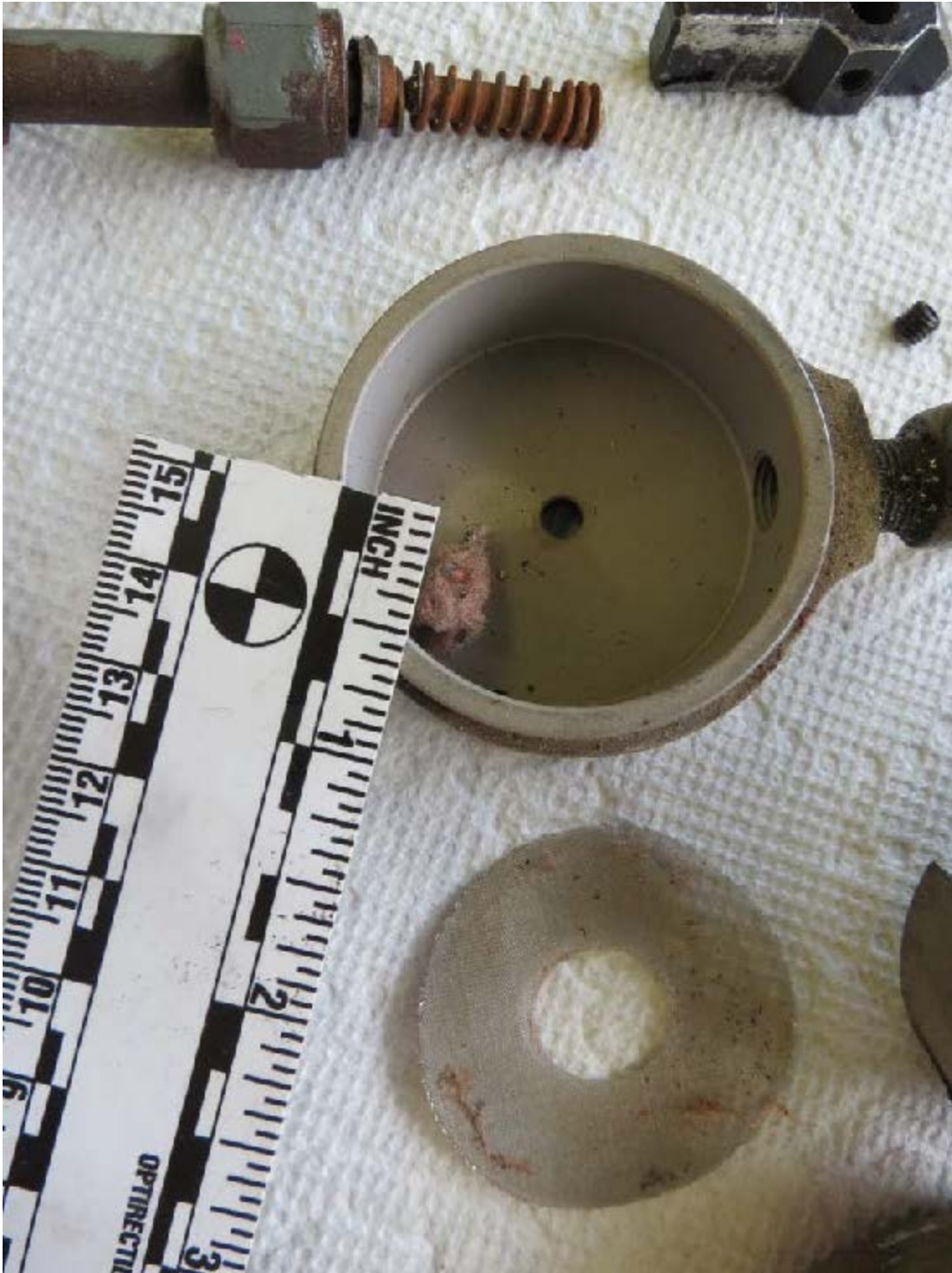
Figure 1-Debris discovered in the fuel selector.
