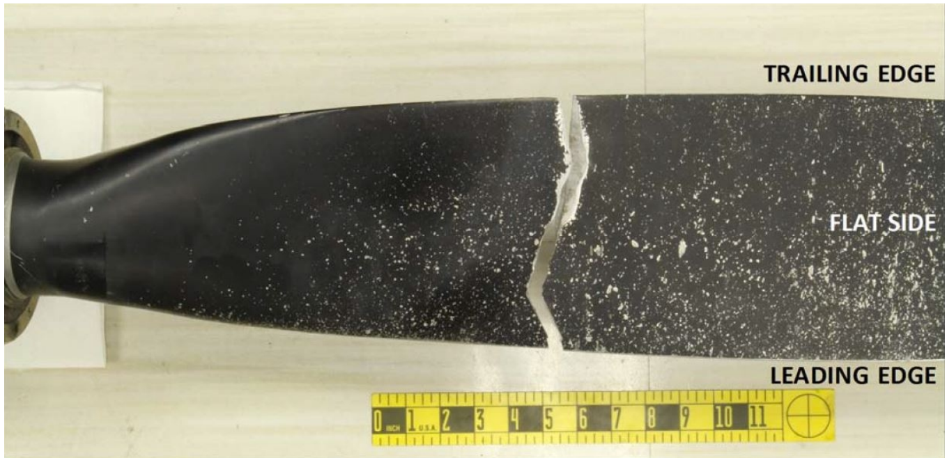
Figure 3 – View of the separated blade (blade #2).
