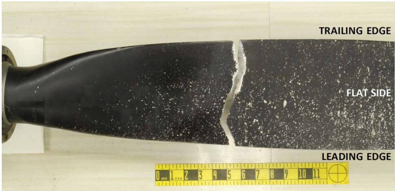
Figure 3 – View of the separated blade (blade #2).
