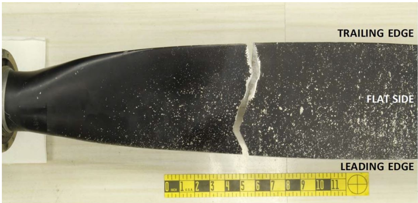
Figure 3 – View of the separated blade (blade #2).
