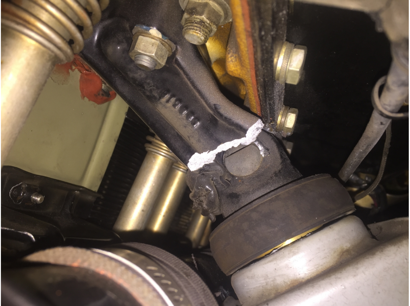
Figure 2 – View of the fractured engine mount (courtesy of the pilot).
