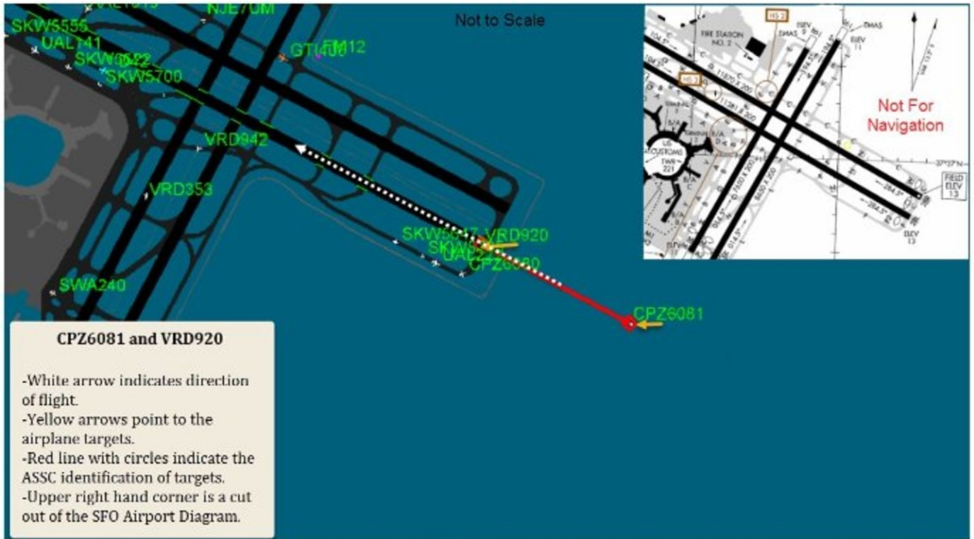
Figure 1. ASSC display screenshot illustrating the position of VRD920 and CPZ6081 when the SFO local controller issued go around instructions.
