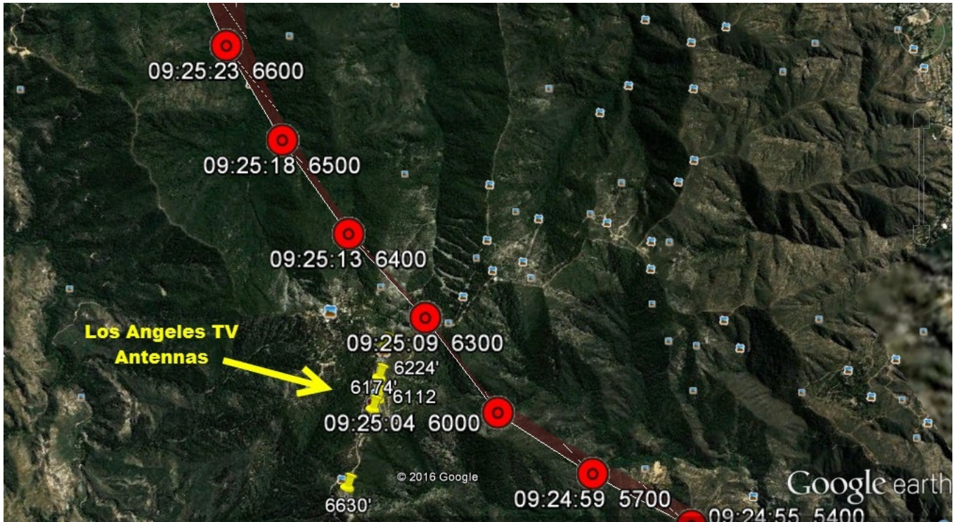
Figure 4 - Radar data overlaid on a Google Earth image with the TV antennas and the associated heights plotted.
