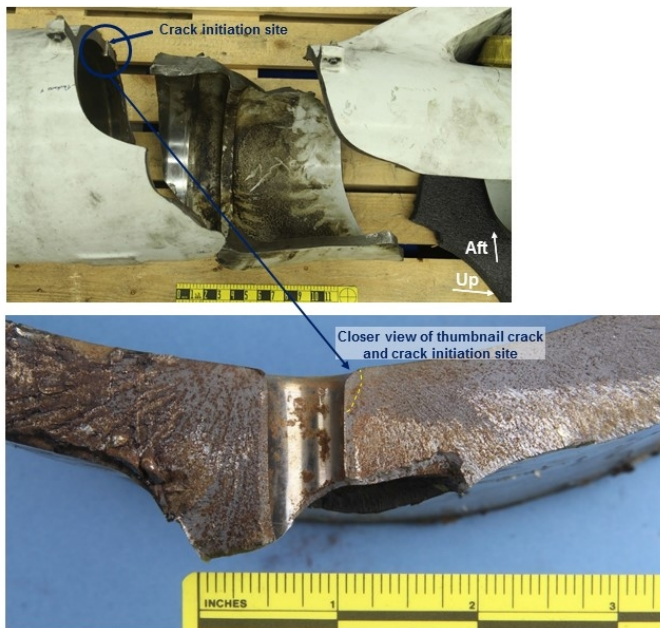
Figure 1. A diagram of an MD-10-10F left MLG (A), photograph of the 3-by-3-inch fragment from the lower section of the accident left MLG cylinder (B), and closer view of the region pointed out in image B (C).
