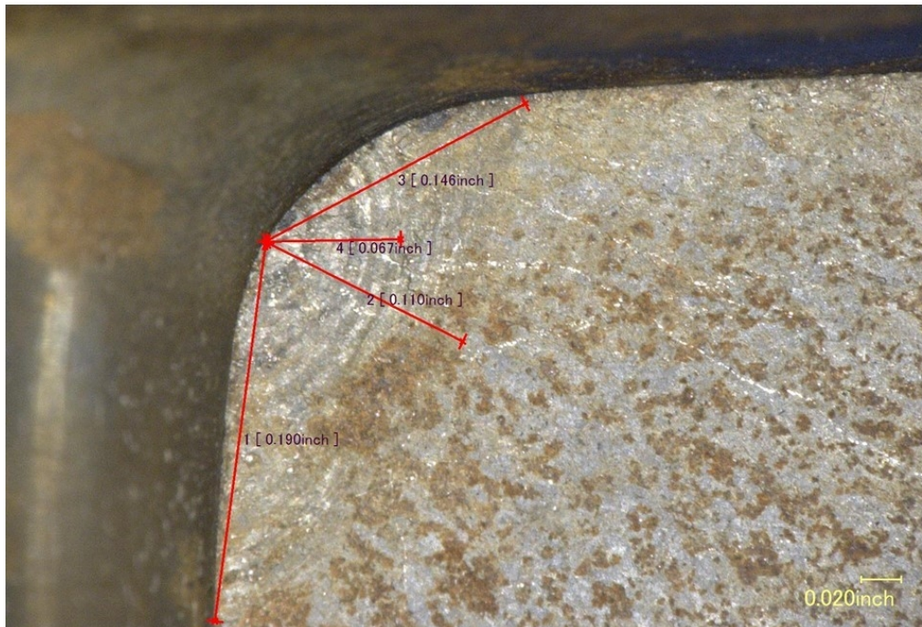
Figure 4. A closeup view of the fatigue striation region.
