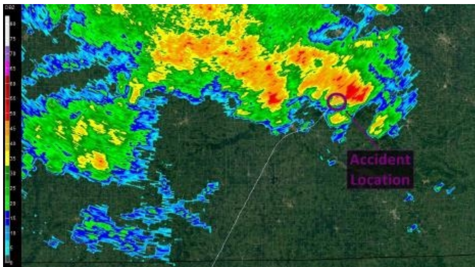
Figure 2. Level-II reflectivity product from a sweep initiated at 1223:06 CDT. Accident flight path through the accident time denoted by white line with accident location marked.
