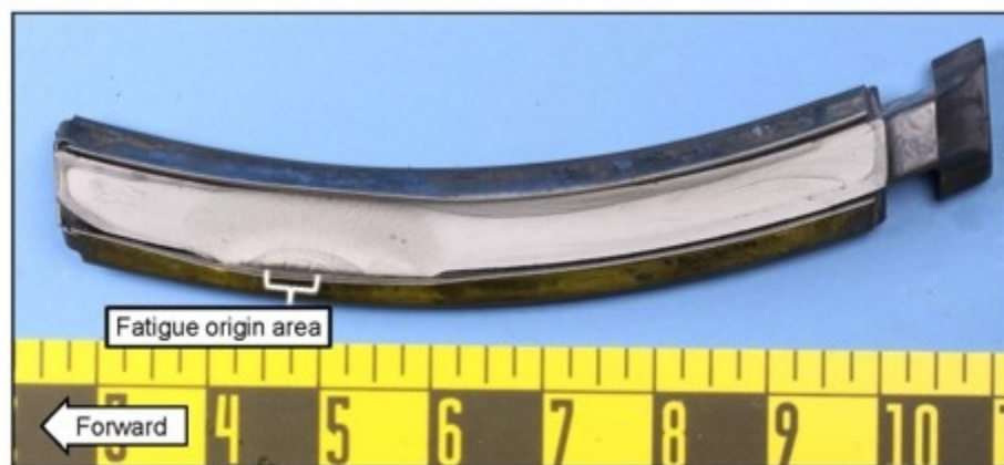
Figure 7. Fan blade No. 23 fracture surface.
