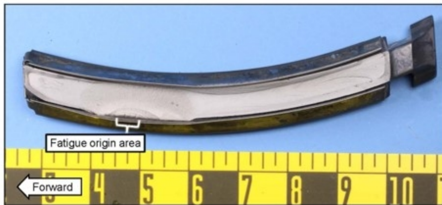
Figure 7. Fan blade No. 23 fracture surface.
