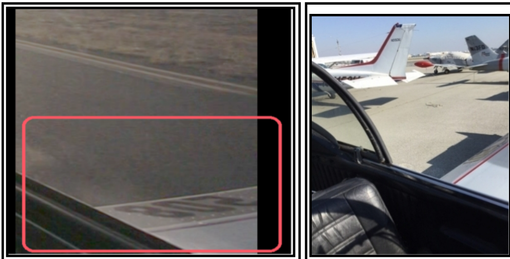
takeoff flap position. Figure 2: Exemplar airplane's flaps set to takeoff position.
