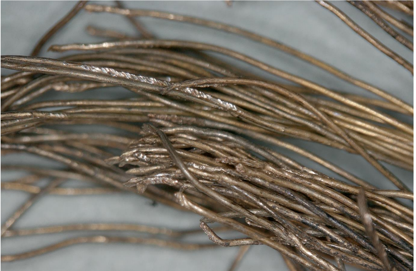
Figure 3 - Photograph of fractured end of L Main 2
