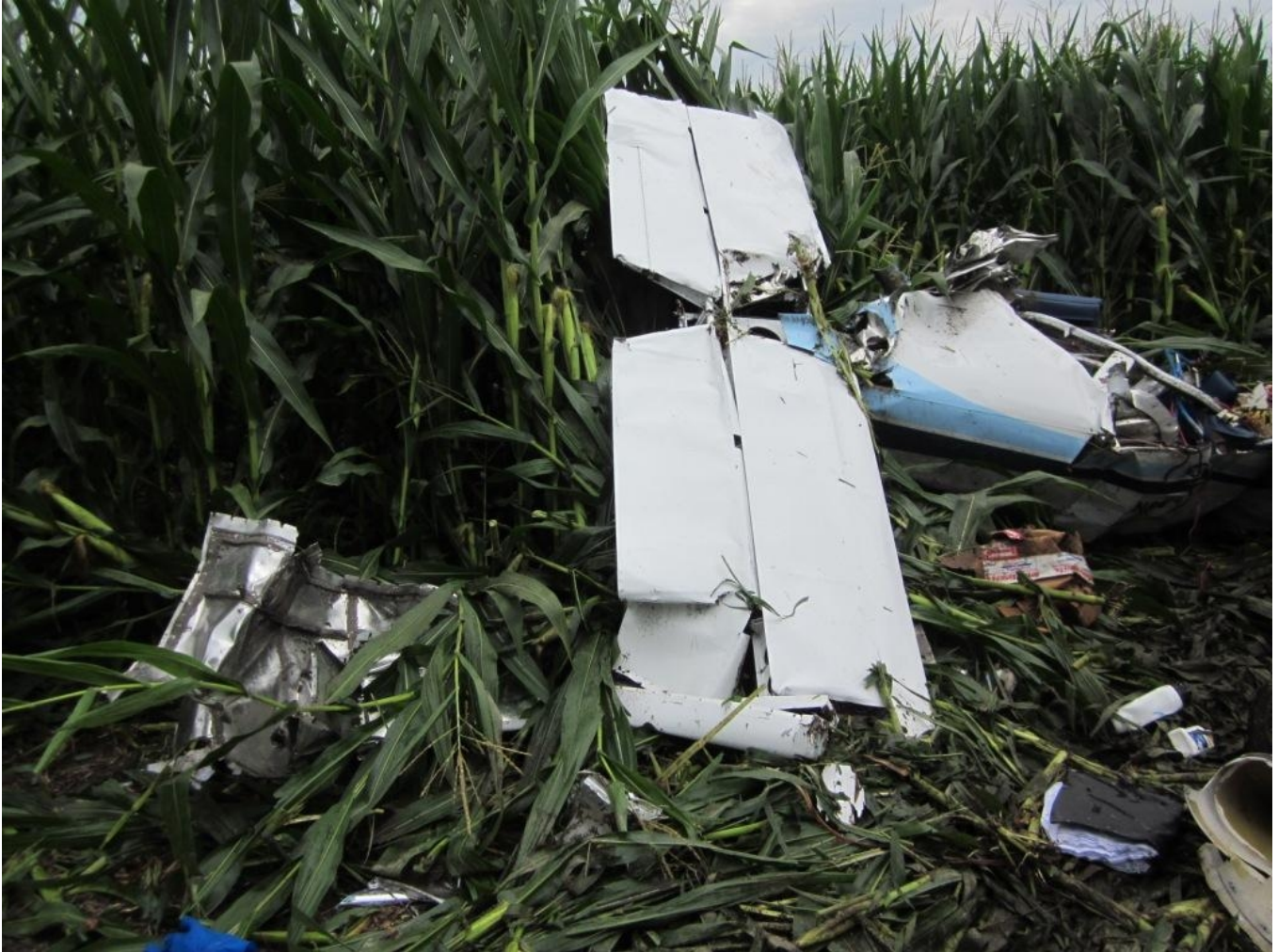
Figure 4 – Right side view of the main wreckage in a mature corn field. The vertical stabilizer and rudder are missing from the empennage.
