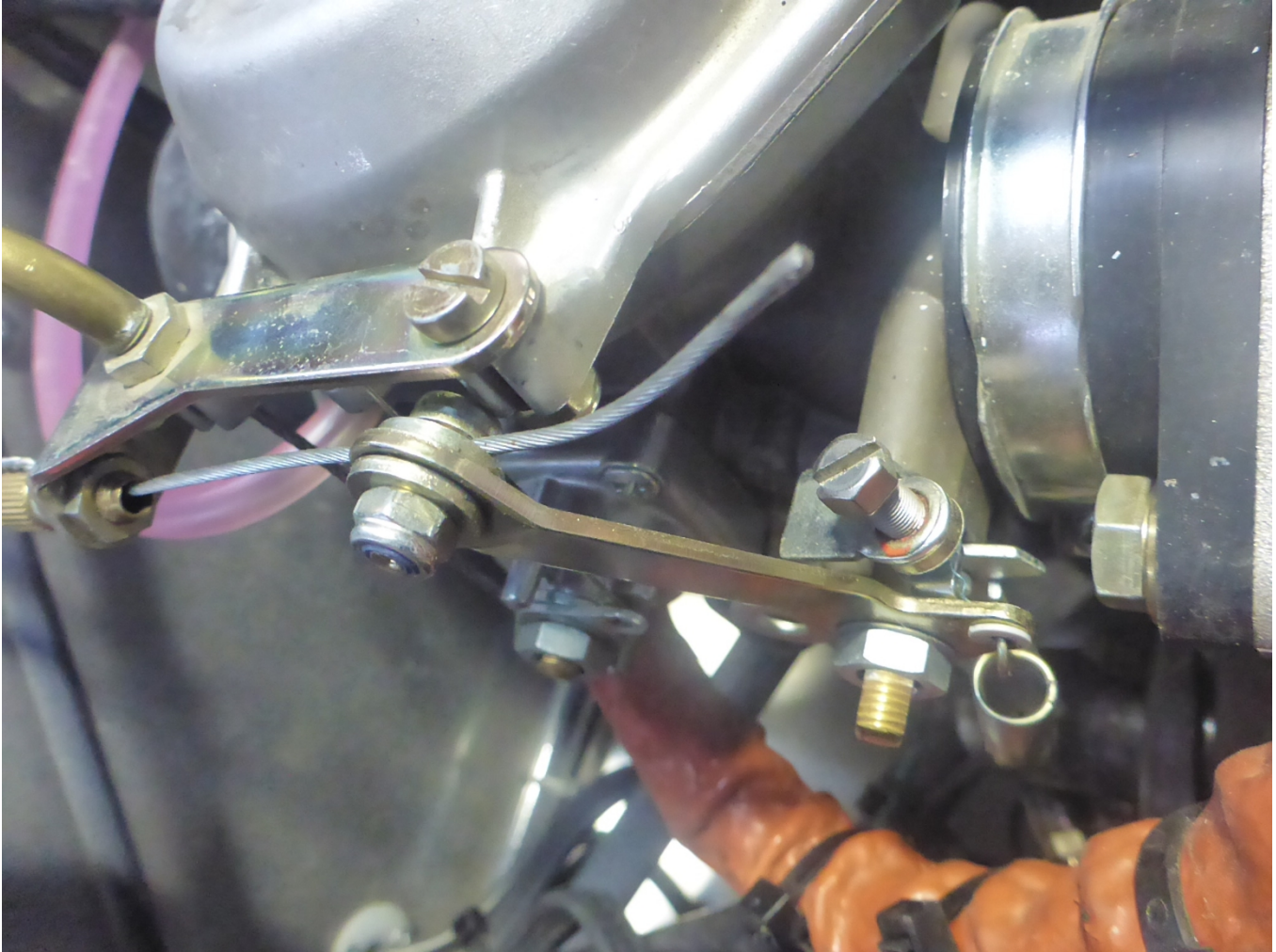
Figure 1: 1/3 carburetor contacting the chamber top
