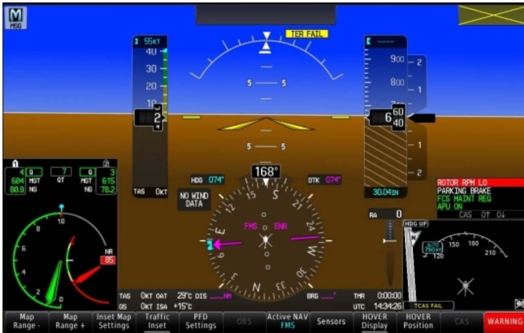
Figure 6. Example of PFD during "ROTOR RPM LO" warning.
