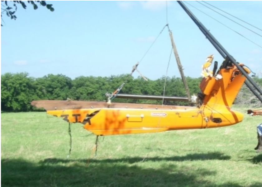
Figure 8. Angled cut line at the forward end of the aft section of the tail boom.
