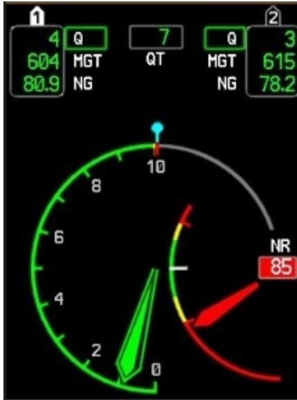
Figure 4. PSI displaying Nr as an arc.
