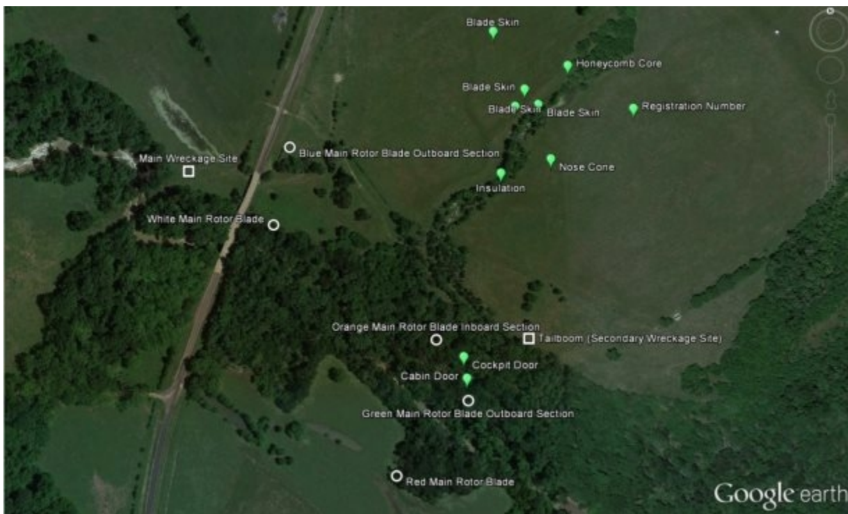
Figure 7. The location of the main wreckage site, secondary wreckage site, and selected items from the wreckage debris field.
