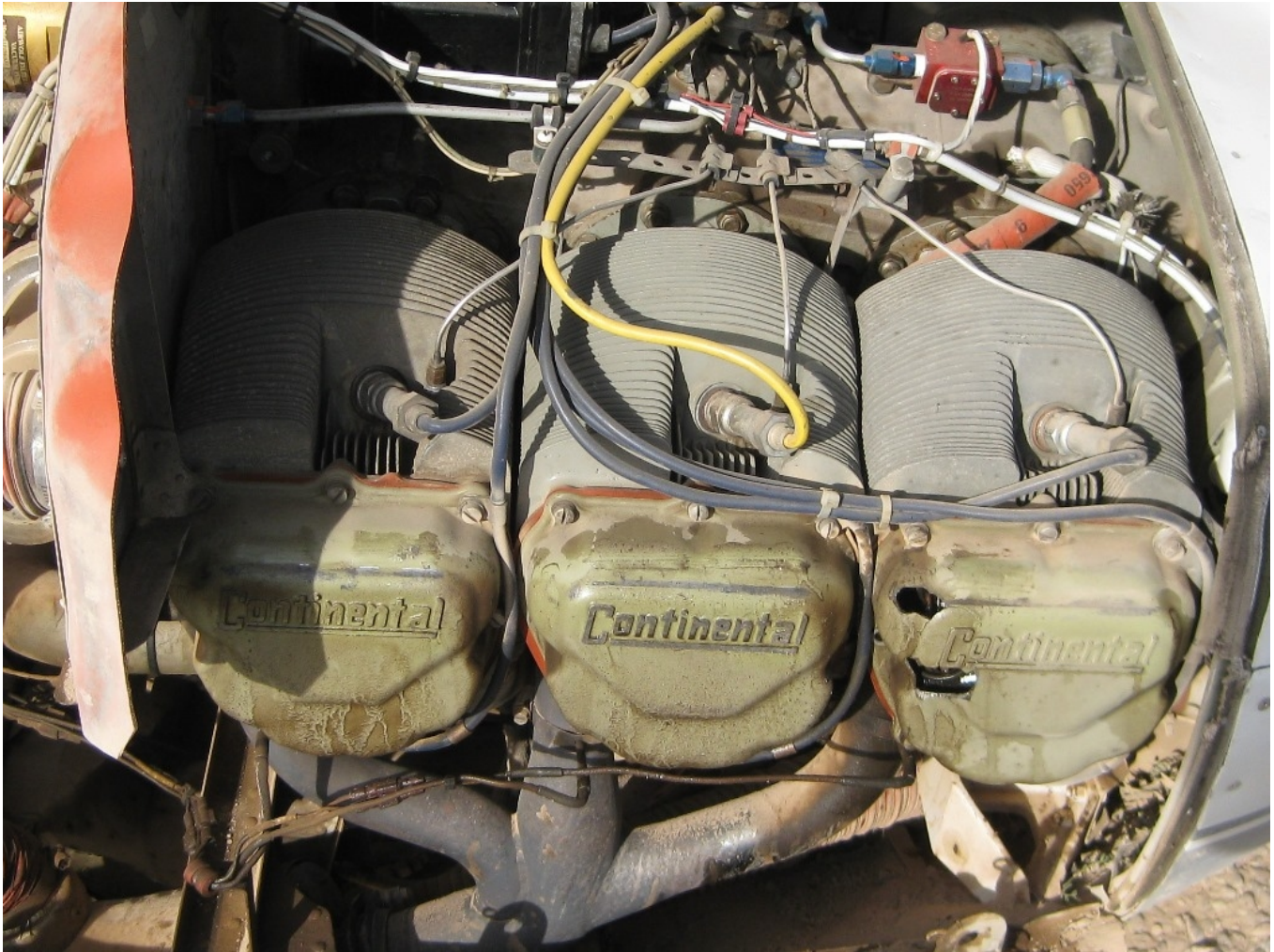
Figure 3 – Engine Cylinder No. 5 Damage
