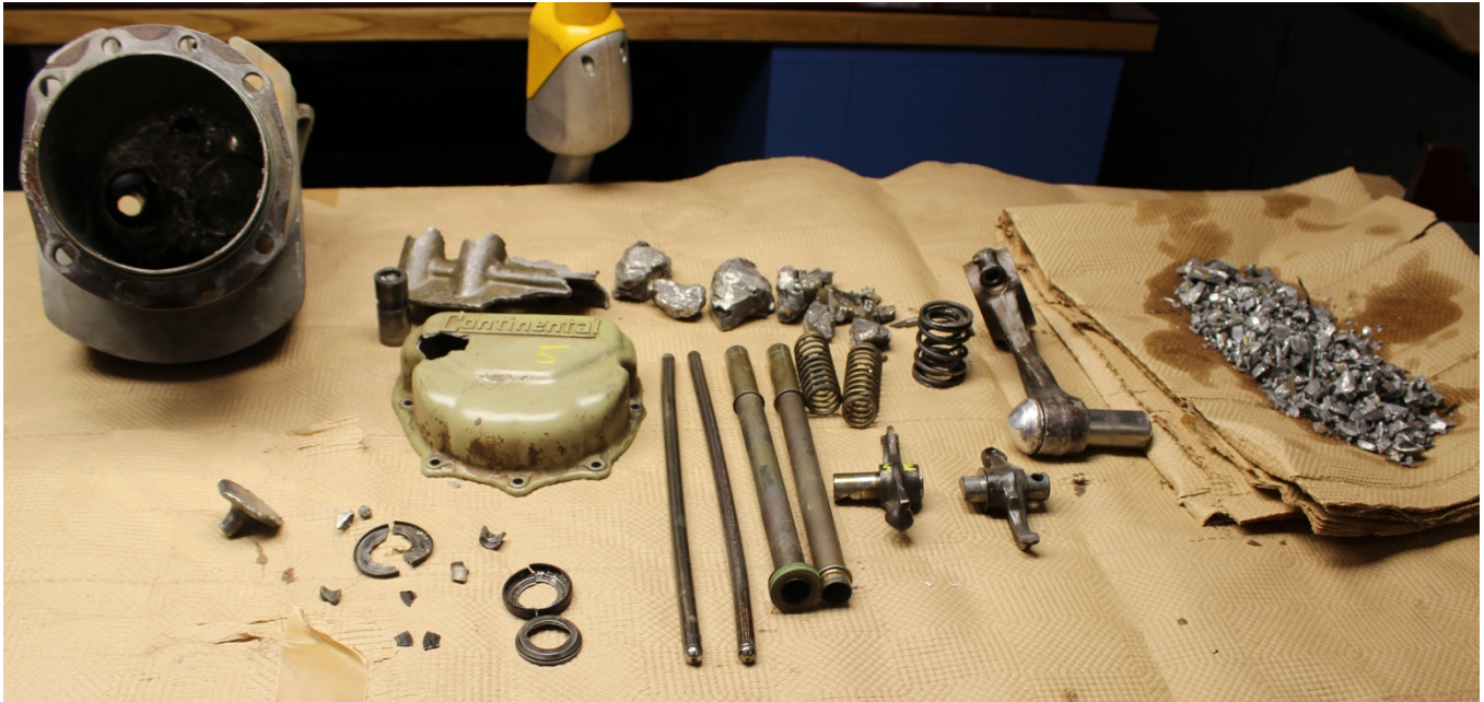
Figure 4 – No. 5 Cylinder Parts Disassembled
