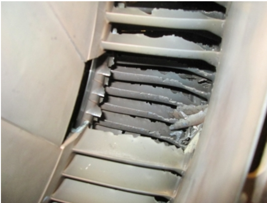
Photo No. 1: View of missing 3rd stage turbine vane cluster from front of LPT. (Delta)
