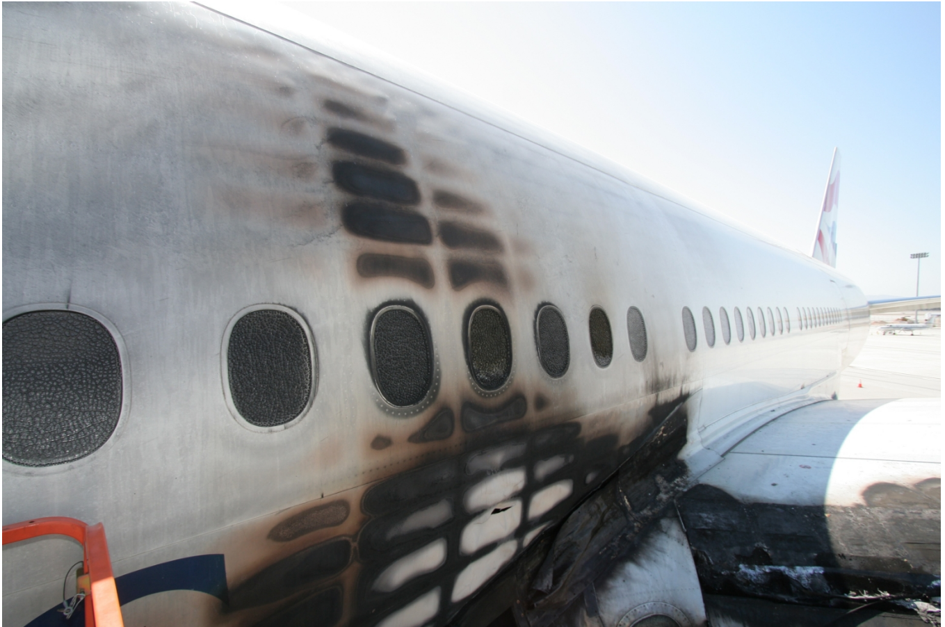
Figure 3. Thermally damaged fuselage skin and thermally crazed windows
