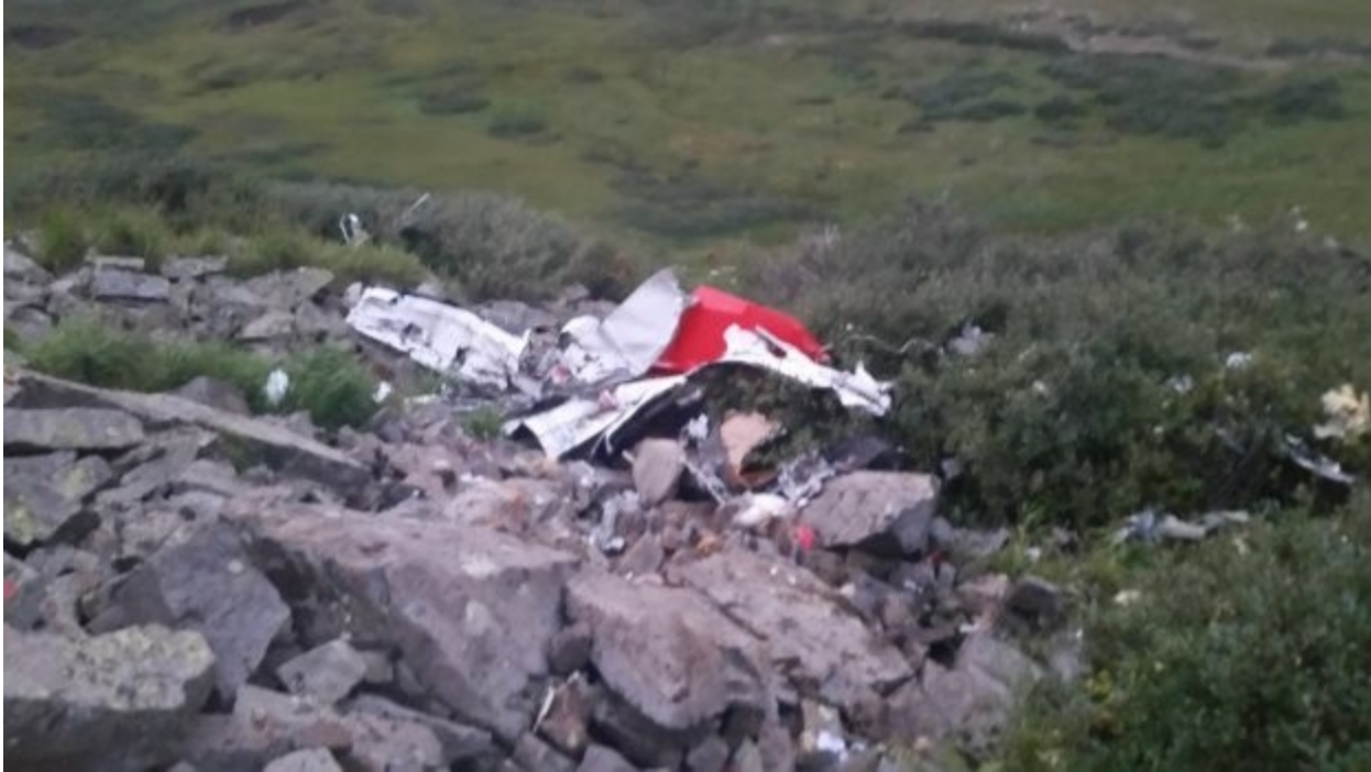
Figure 5. A photograph of the main wreckage, which was destroyed by impact forces with no evidence of soot or fire. The airplane wings, horizontal and vertical stabilizers, engines, and propellers were located at accident site.
