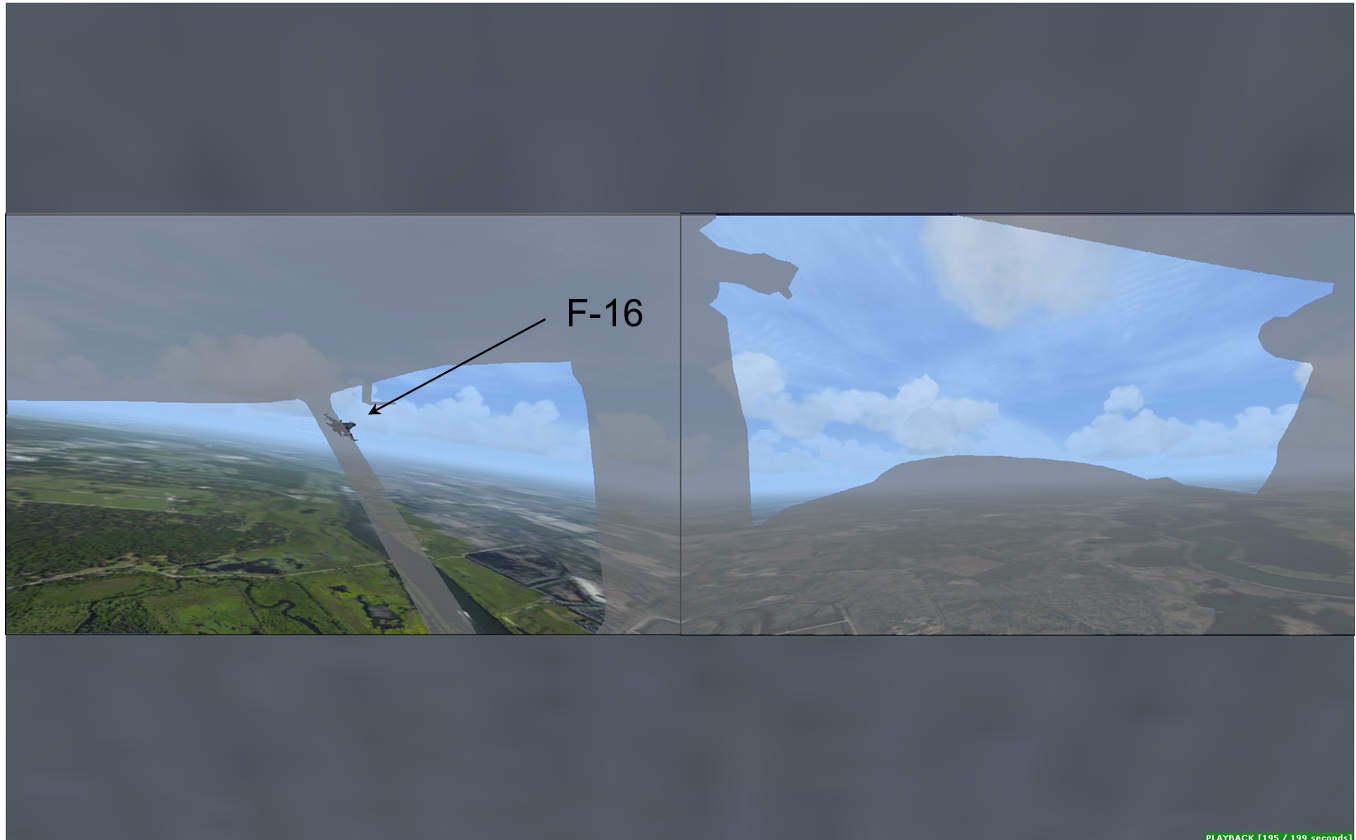
Figure 5b. Simulated cockpit visibility from the Cessna at 1100:56, when the airplanes were 260 ft apart.
