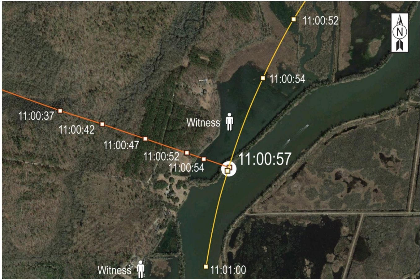
Figure 1. Calculated flight track for the F-16 (yellow) and the Cessna (orange). (The first witness is located north of the collision point, and the second witness is located southwest of the collision point.)
