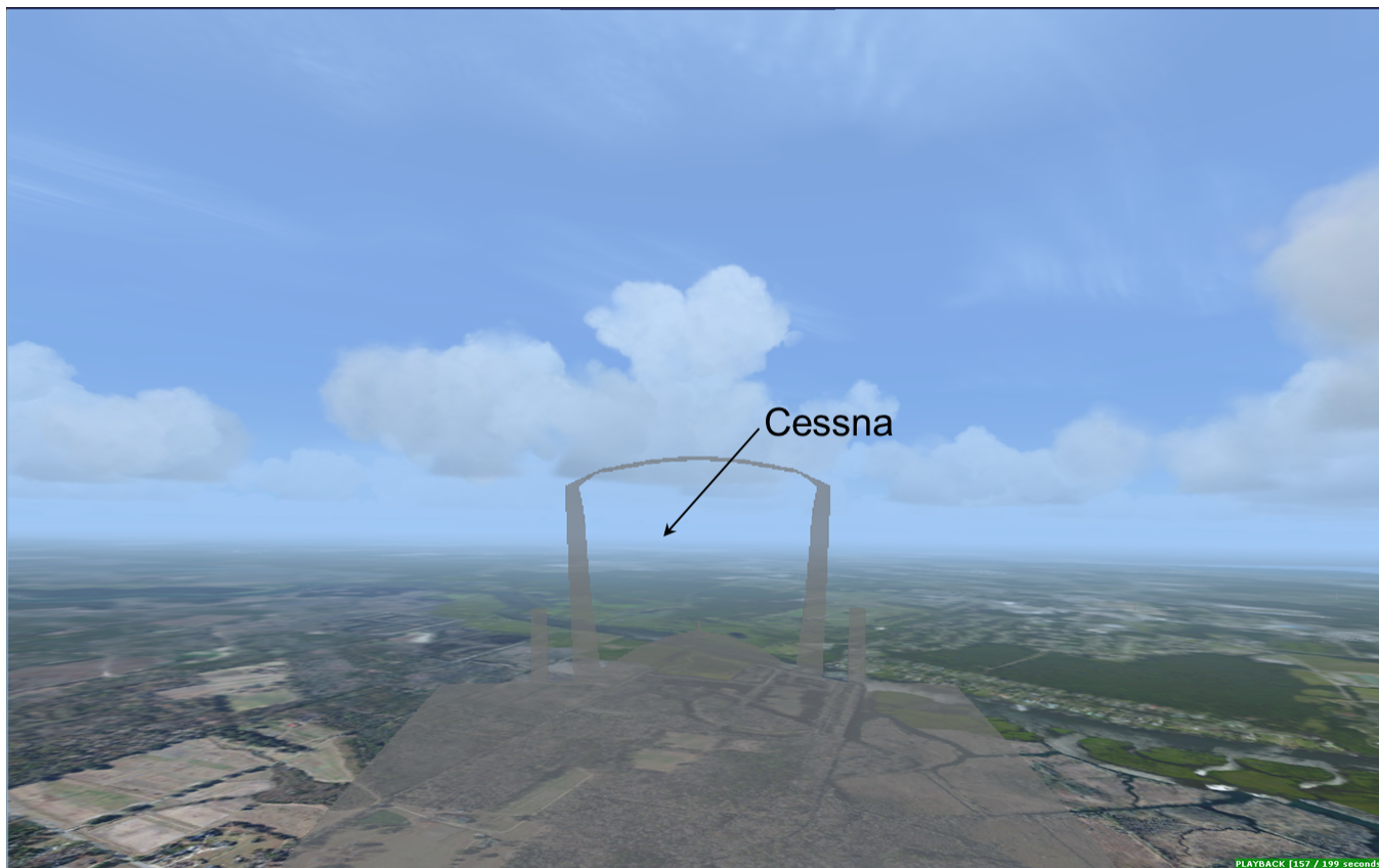
Figure 3a. Simulated cockpit visibility from the F-16 at 1100:18, when the airplanes were 3.1 nm apart.
