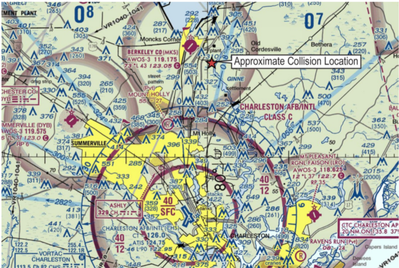
Figure 2. FAA sectional aeronautical chart view depicting CHS and class C airspace, MKS, and the approximate collision location. (Not for navigational use.)
