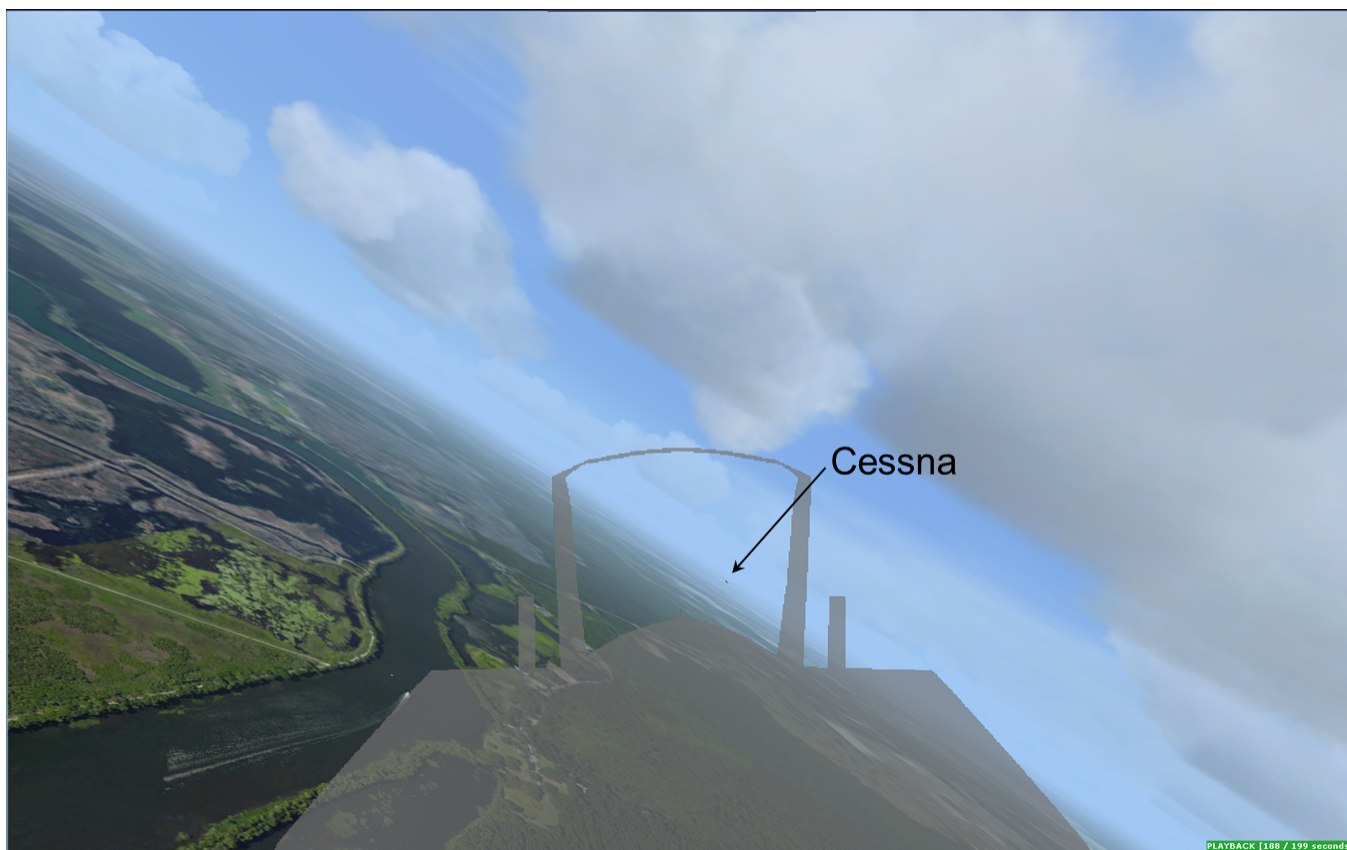
Figure 4a. Simulated cockpit visibility from the F-16 at 1100:49, when the airplanes were 0.6 nm apart.
