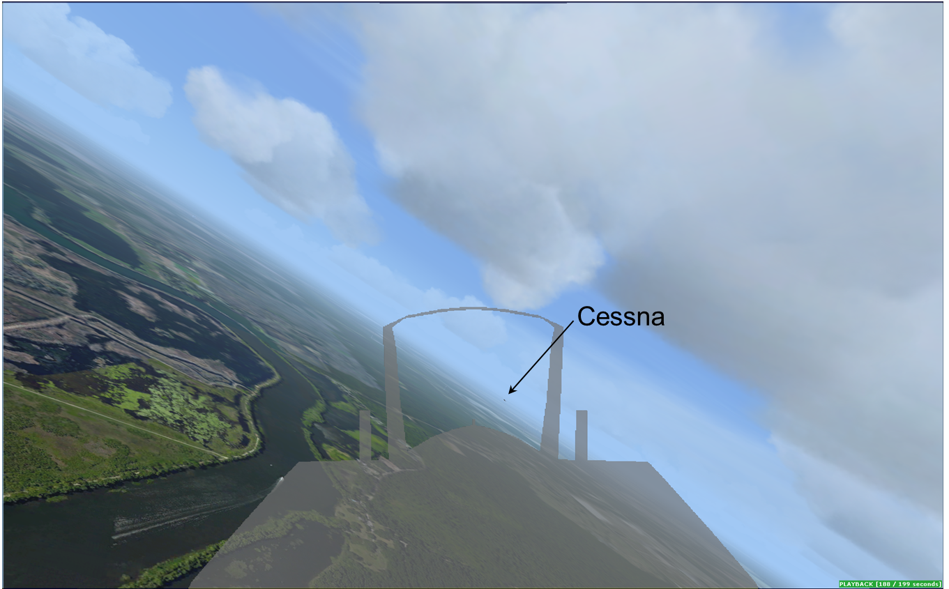
Figure 4a. Simulated cockpit visibility from the F-16 at 1100:49, when the airplanes were 0.6 nm apart.
