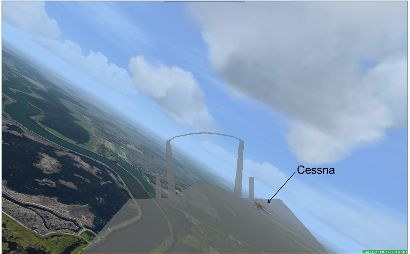
Figure 5a. Simulated cockpit visibility from the F-16 at 1100:56, when the airplanes were 260 ft apart.
