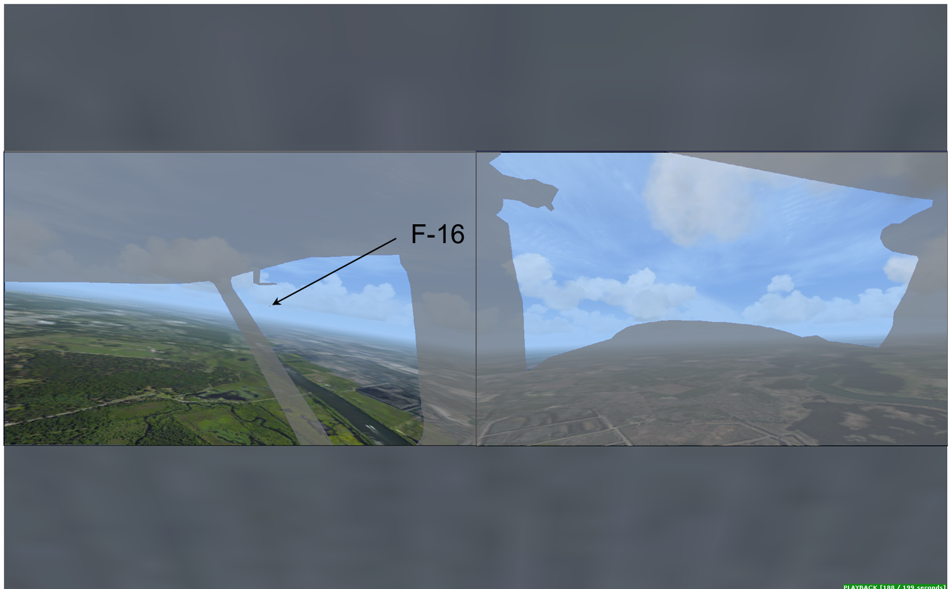
Figure 4b. Simulated cockpit visibility from the Cessna at 1100:49, when the airplanes were 0.6 nm apart.
