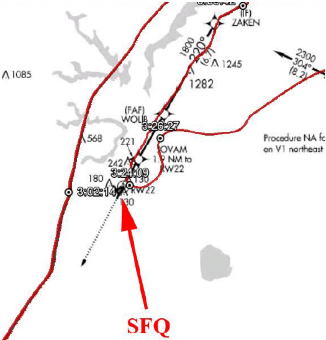
Figure 2 - The airplane's GPS-derived ground track overlaid onto the SFQ RNAV GPS 22 instrument approach procedure plan view.
