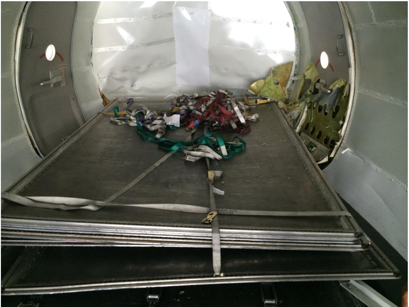
Figure 1: Pallet cookie sheets and damage to aft pressure bulkhead
