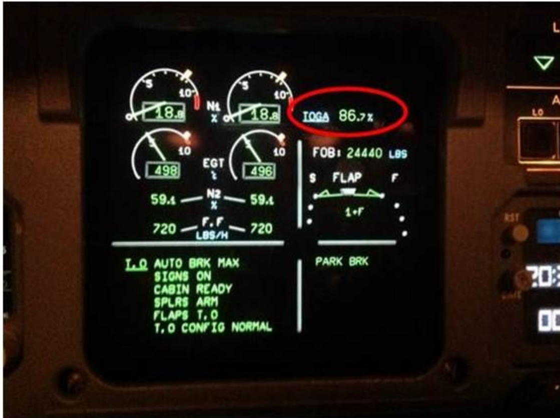
Figure 4. Upper ECAM without FLEX temperature inserted in MCDU (TO/GA indicated).
